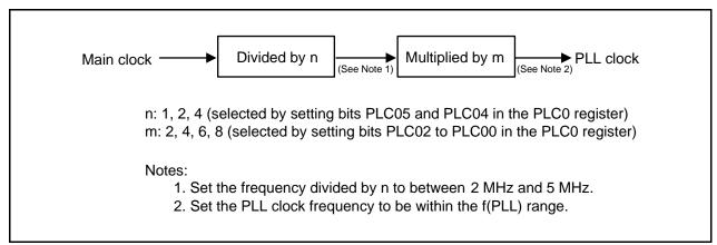
Figure 8.3 Relation between Main Clock and PLL Clock
