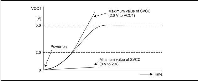
Figure 32.2 SVCC Timing (3.6 V < VCC1)
