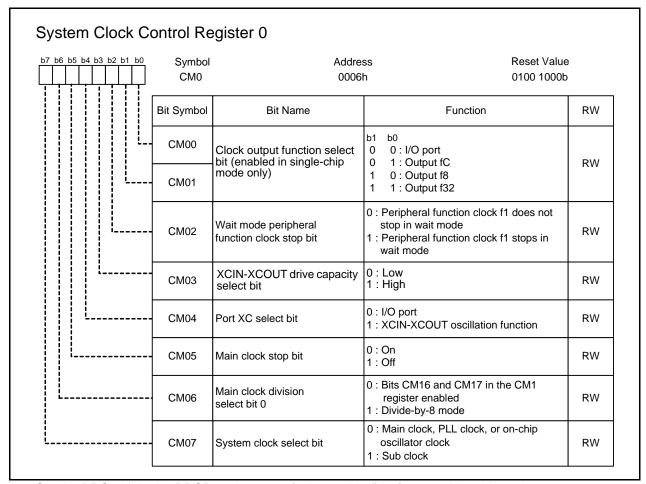
Set the PRC0 bit in the PRCR register to 1 (write enabled) before rewriting this register. See Table 9.3 "Clock-Related Bit Setting and Modes" to select a clock and mode.
