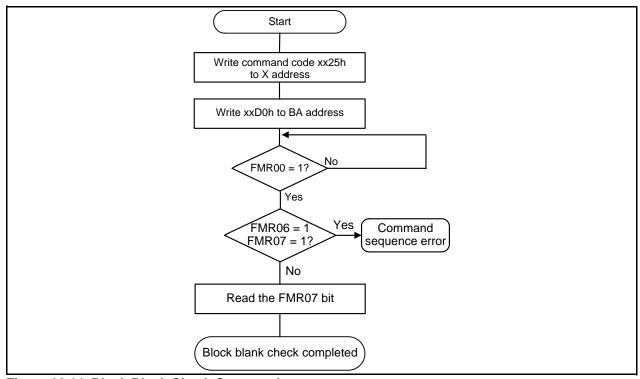
Figure 30.14 Block Blank Check Command
