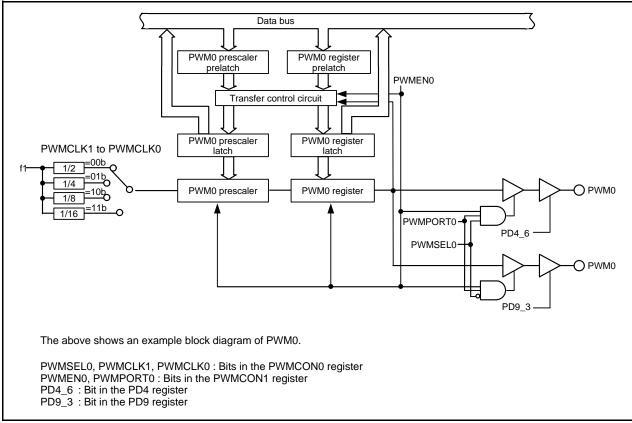
Figure 21.1 Block Diagram of PWM
