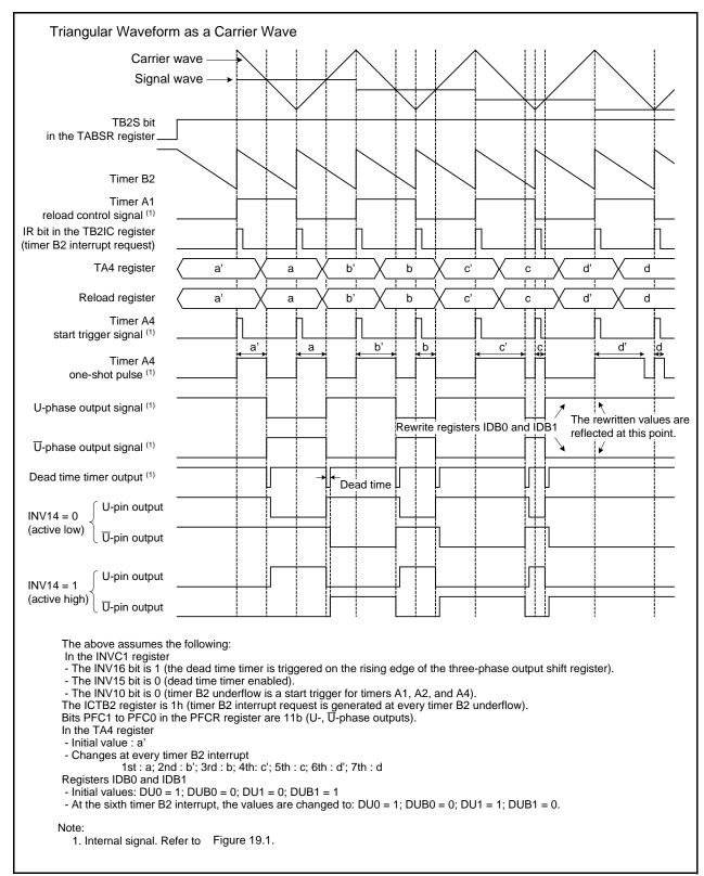
Figure 19.6 Example of Three-Phase Mode 0 Operation
