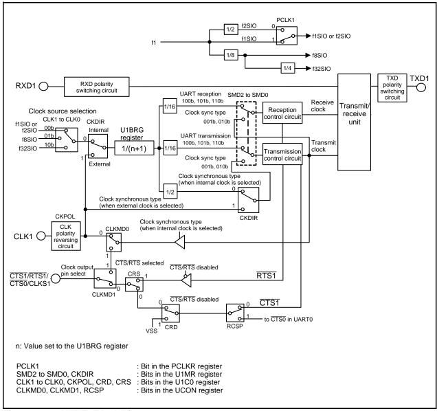
Figure 23.2 UART1 Block Diagram
