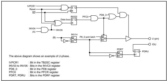
Figure 19.2 Three-Phase Motor Control Timer Function Block Diagram 2
