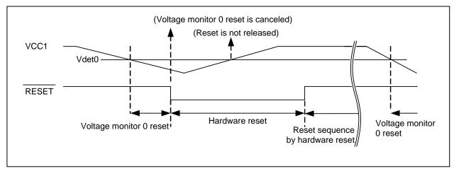
Figure 32.4 Hardware Reset when VCC1 < Vdet0
