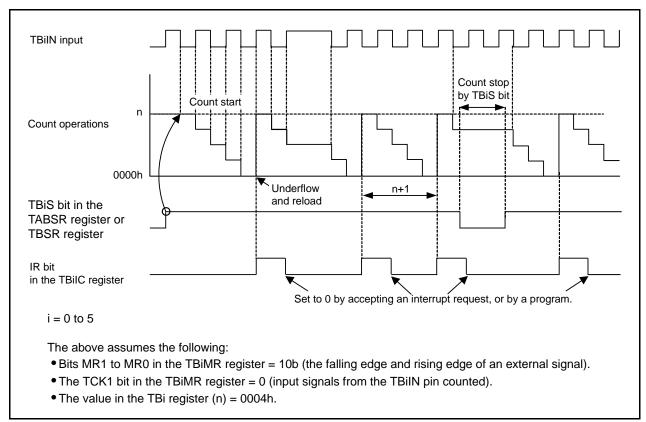
Figure 18.5 Operation Example in Event Counter Mode
