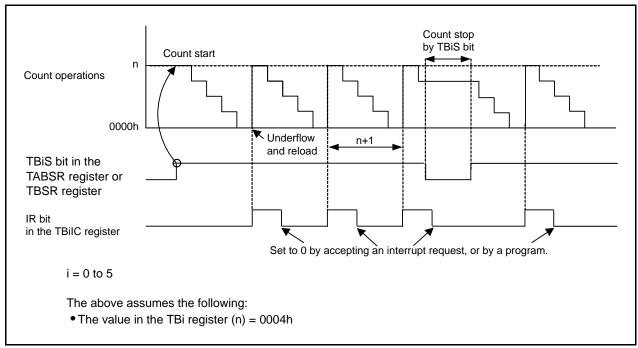
Figure 18.4 Operation Example in Timer Mode
