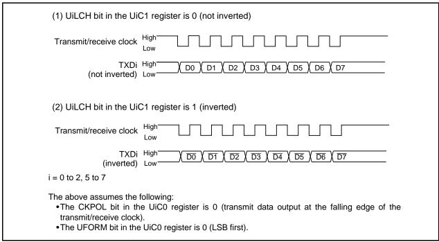
Figure 23.9 Serial Data Logic
