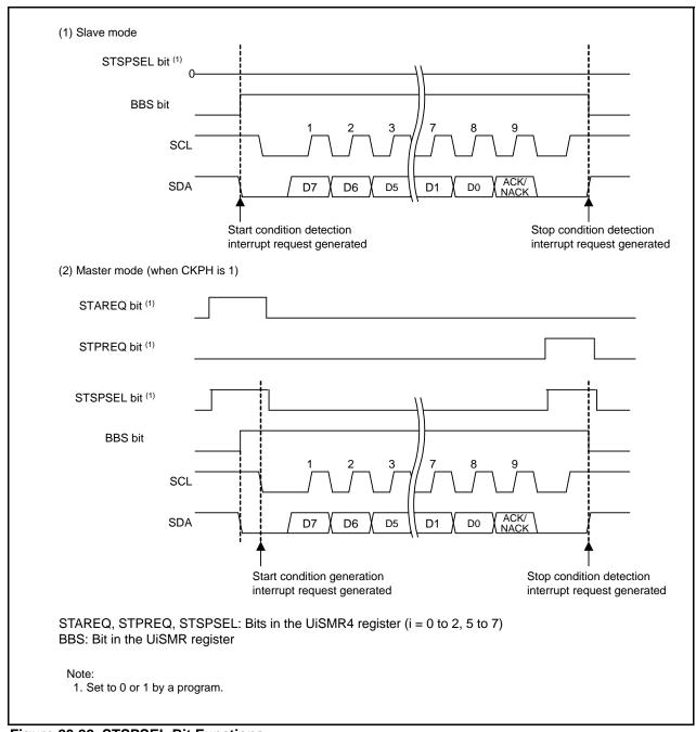
Figure 23.22 STSPSEL Bit Functions
