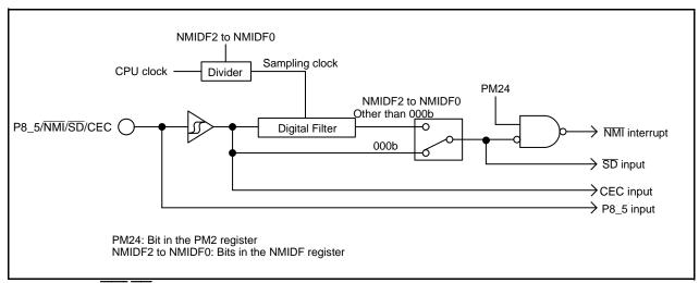
Figure 13.13 NMI/SD Digital Filter
