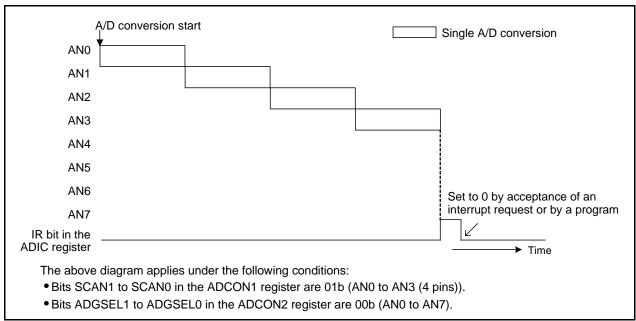
Figure 27.12 Operation Example in Single Sweep Mode
