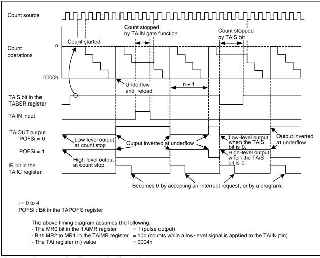
Figure 17.5 Operation Example in Timer Mode
