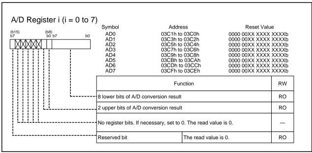
The A/D conversion result is stored in the ADi register corresponding to pins ANi, ANEXi, AN0\_i, and AN2\_i. Read the ADi register in 16-bit units. Table 27.4 lists Analog Pin and A/D Conversion Result Storing Register.
