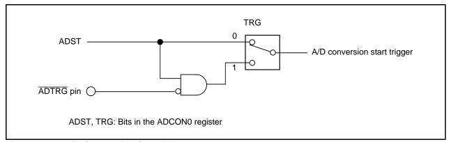
Figure 27.4 A/D Conversion Start Trigger
