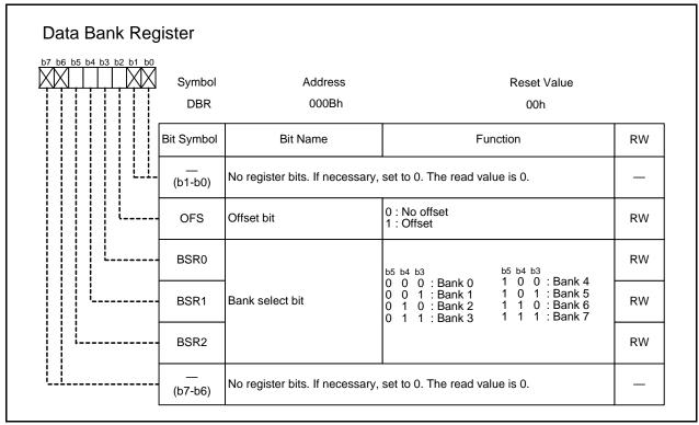
The DBR register is enabled when bits PM01 to PM00 in the PM0 register are 01b (memory expansion mode) or 11b (microprocessor mode).
