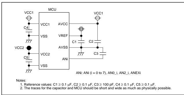
Figure 32.16 Example of Pin Configuration
