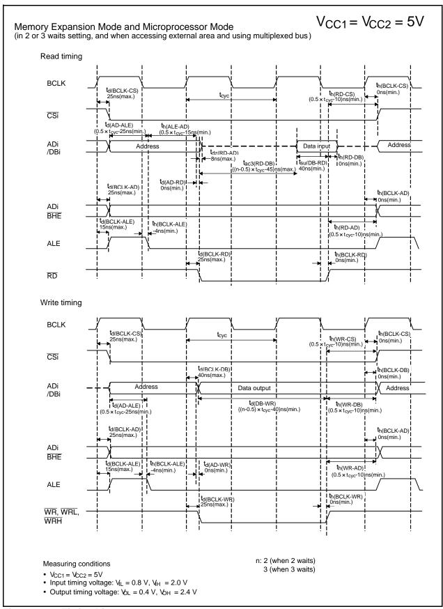
Figure 31.17 Timing Diagram
