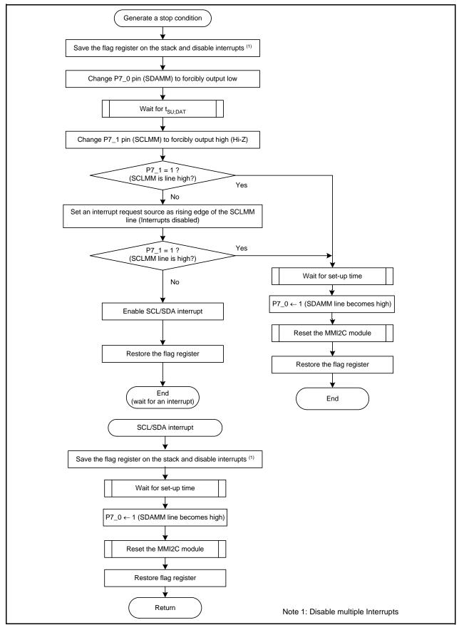
Figure 32.14 Generating a Stop Condition
