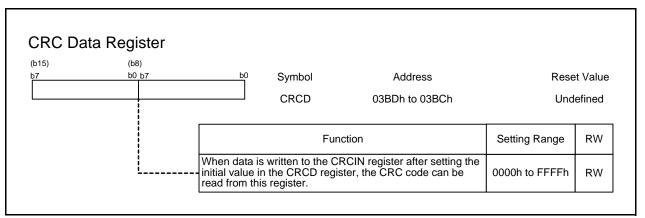
Write 0000h to the CRCD register and then write the first data to the CRCIN register. Execute this operation every time CRC calculation is performed. Refer to the setting procedures described in Figure 29.2 "CRC Calculation When Using CRC-CCITT" and Figure 29.3 "CRC Calculation When Using CRC-16".
