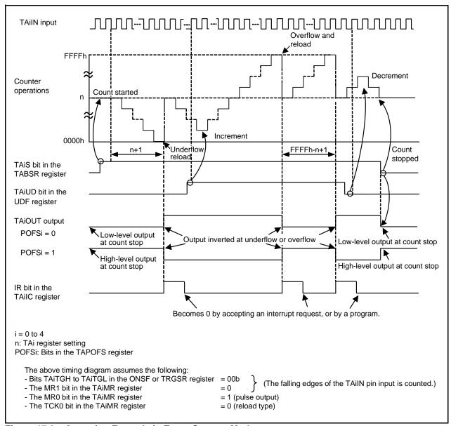
Figure 17.6 Operation Example in Event Counter Mode
