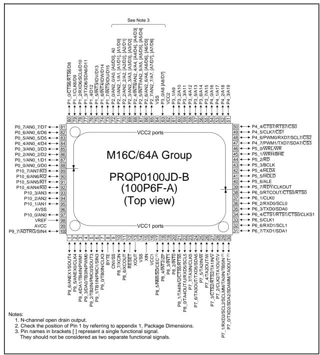
Figure 1.4 Pin Assignment for the 100-Pin Package
