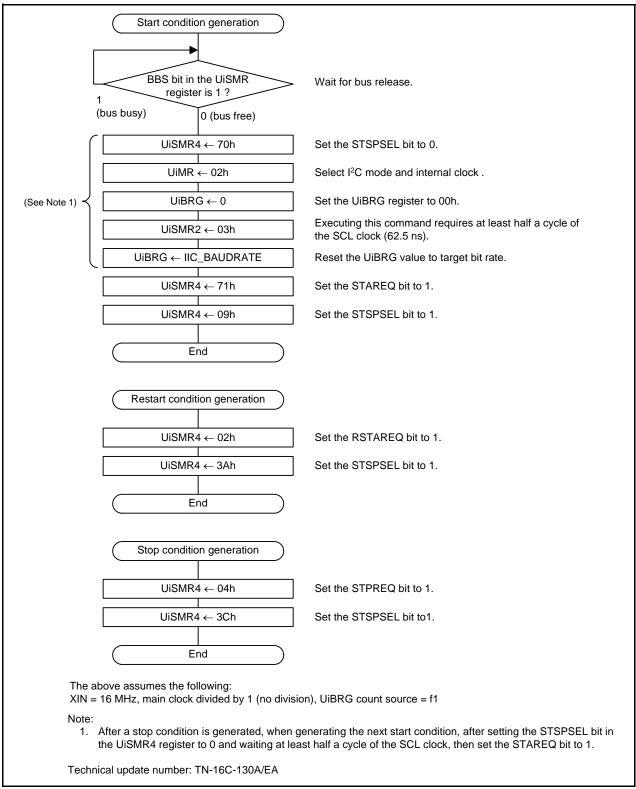
Figure 23.23 Register Setting Procedures for Condition Generation
