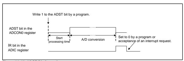
Figure 32.17 ADST Bit Operation
