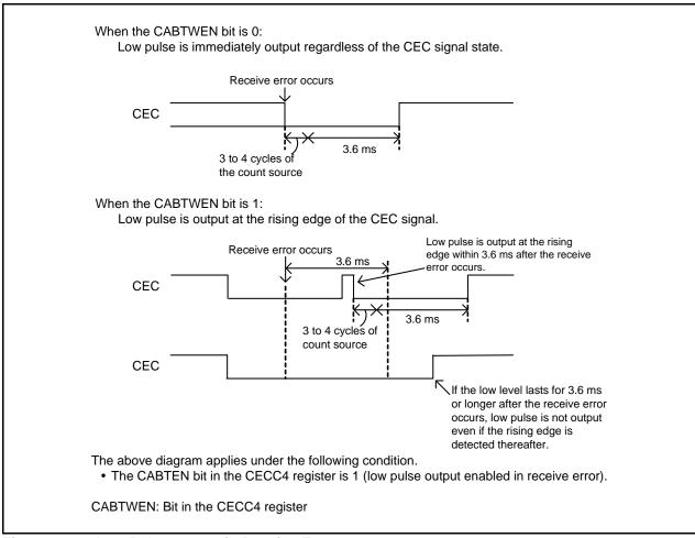
Figure 26.8 Low Pulse Output in Receive Error
