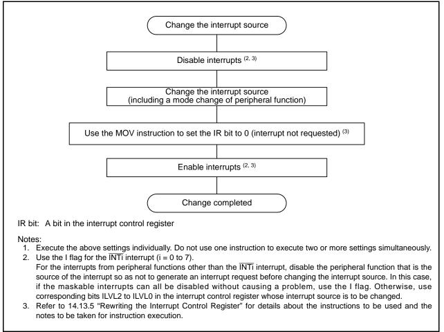
Figure 14.12 Procedure for Changing the Interrupt Generate Source
