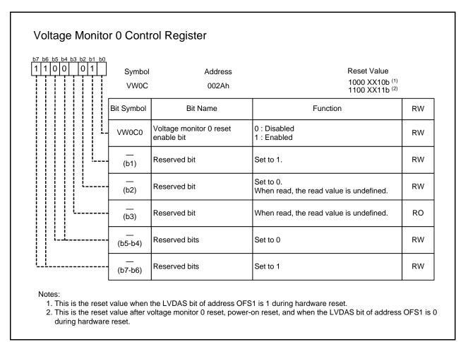
Set the PRC3 bit in the PRCR register to 1 (write enabled) before rewriting to this register.
