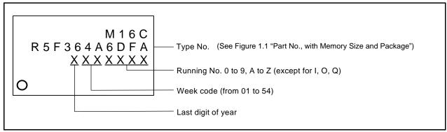
Figure 1.2 Marking Diagram (Top View)
