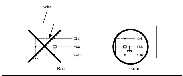
Figure 8.8 Clock I/O Pin Wiring
