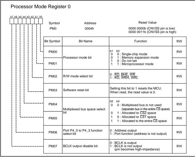
Write to this register after setting the PRC1 bit in the PRCR register to 1 (write enabled).
