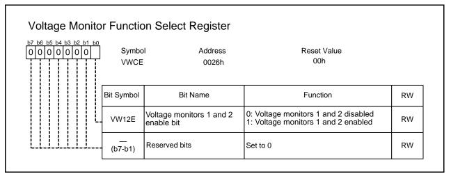
Set the PRC3 bit in the PRCR register to 1 (write enabled) before rewriting this register.
