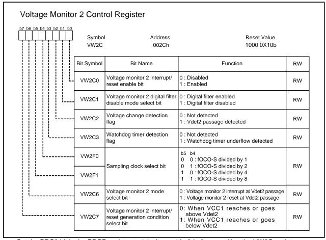
Set the PRC3 bit in the PRCR register to 1 (write enabled) before rewriting the VW2C register.
