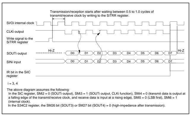
Figure 24.4 SI/Oi Operation Timing (Internal Clock)
