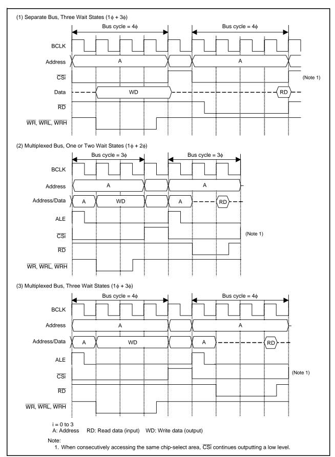
Figure 11.7 Typical Bus Timings Using Software Wait States (2/2)
