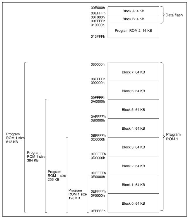
Figure 30.1 Flash Memory Block Diagram
