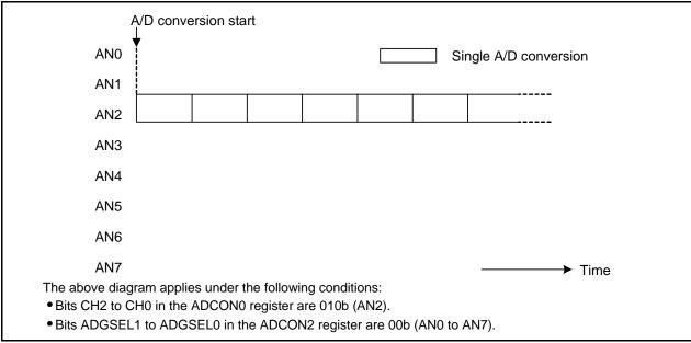
Figure 27.11 Operation Example in Repeat Mode
