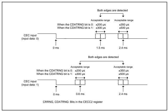
Figure 26.7 Data Bit Acceptable Range (CRRNG Bit = 1)
