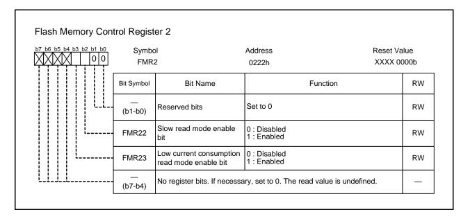
FMR22 (Slow read mode enable bit) (b2) FMR23 (Low-current consumption read mode enable bit) (b3)
