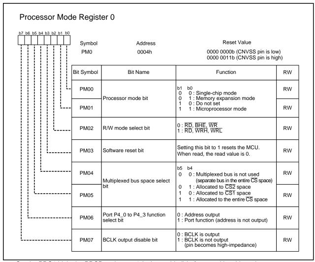
Set the PRC1 bit in the PRCR register to 1 (write enabled) before rewriting this register.
