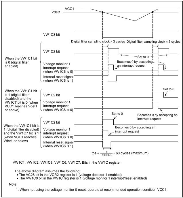
Figure 7.6 Voltage Monitor 1 Interrupt/Reset Operation Example
