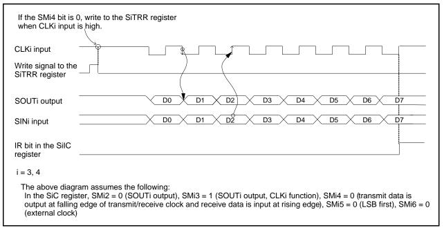
Figure 24.6 SI/Oi Operation Timing (External Clock)
