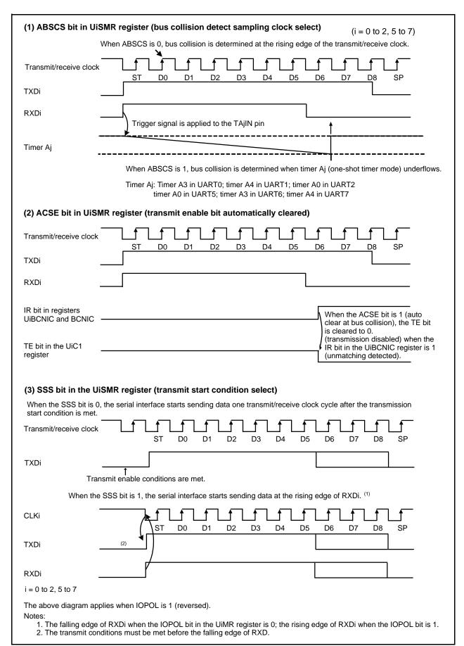
Figure 23.34 Bus Collision Detect Function-Related Bits
