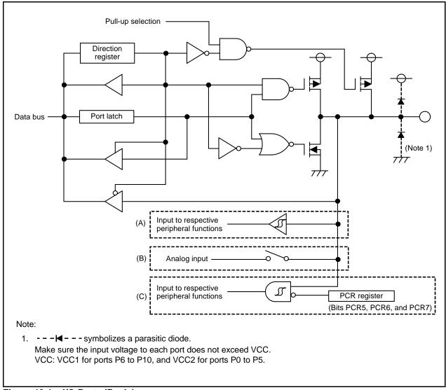
Figure 13.1 I/O Ports (Basic)
