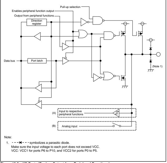
Figure 13.2 I/O Ports (Basic + Output from Peripheral Functions)
