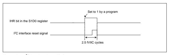
Figure 25.3 I<sup>2</sup>C Interface Reset Timing
