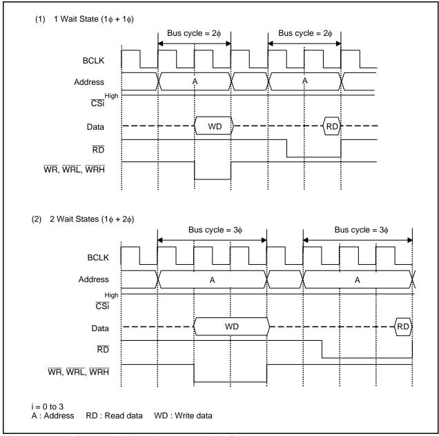
Figure 11.5 Typical Bus Timings When Accessing SFRs
