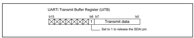
Figure 23.27 UiTB Register Setting (SDA Output)
