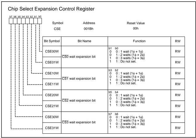
Set the CSiW bit (i = 0 to 3) in the CSR register to 0 (wait state) before writing to bits CSEi1W to CSEi0W. To set the CSiW bit to 1 (no wait state), set bits CSEi1W to CSEi0W to 00b first, and then set the CSiW bit to 1.
