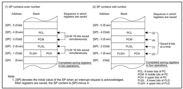
Figure 14.6 Register Save Operation
