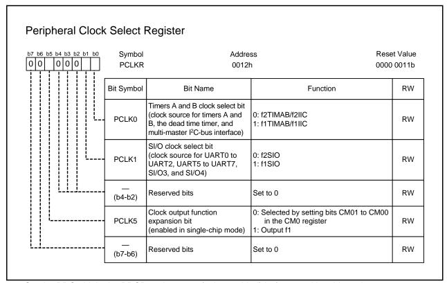
Set the PRC0 bit in the PRCR register to 1 (write enabled) before rewriting this register.
