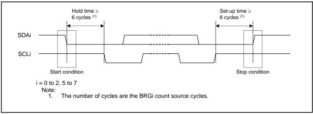
Figure 23.21 Detecting Start and Stop Conditions
