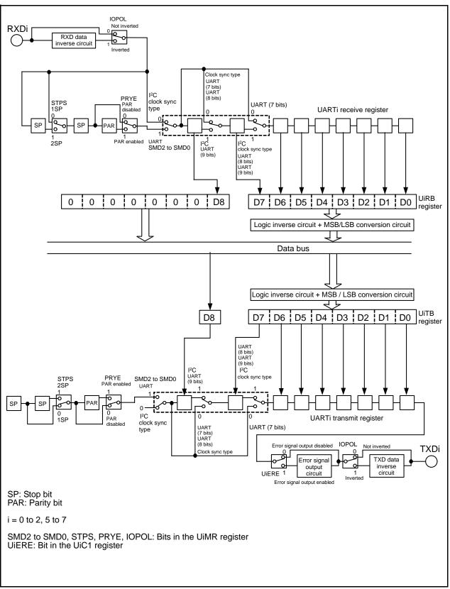
Figure 23.4 UARTi Transmit/Receive Unit Block Diagram
