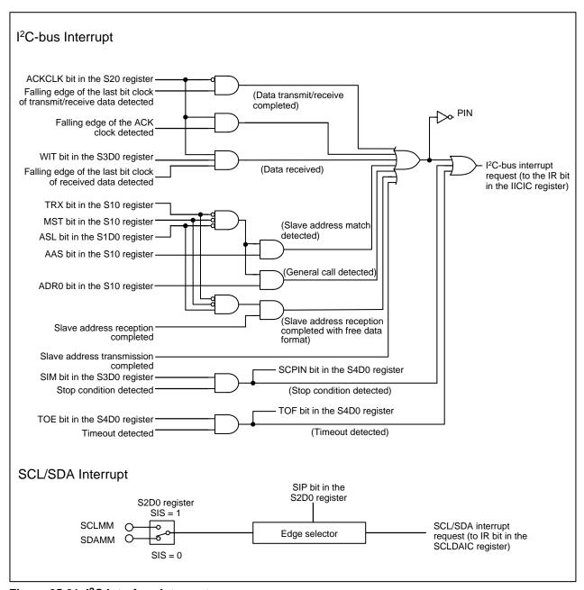
Figure 25.21 I<sup>2</sup>C Interface Interrupts
