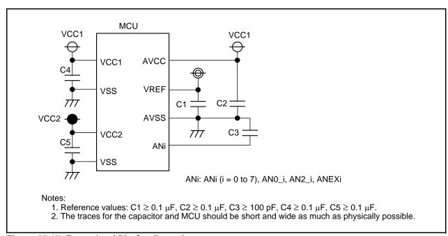
Figure 27.17 Example of Pin Configuration
