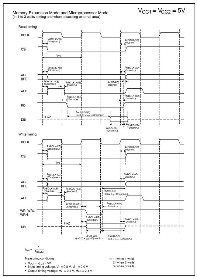
Figure 31.16 Timing Diagram
