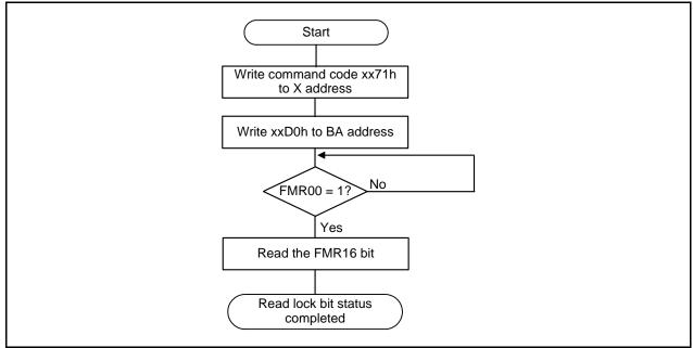
Figure 30.13 Read Lock Bit Status Command
