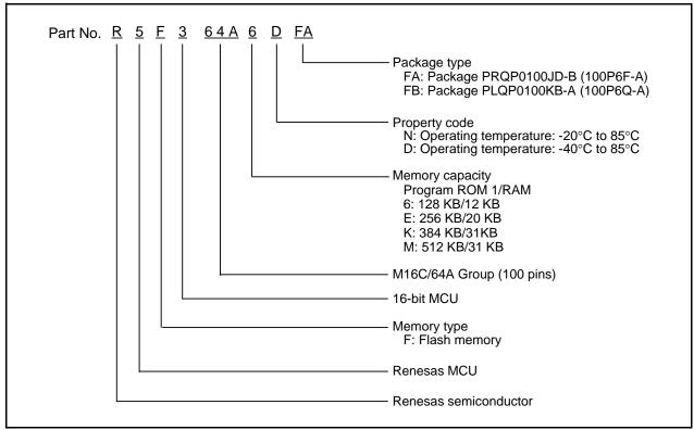
Figure 1.1 Part No., with Memory Size and Package
