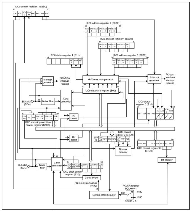
Figure 25.1 Multi-master I<sup>2</sup>C-bus Interface Block Diagram
