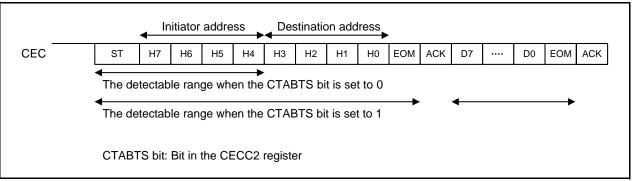
Figure 26.14 Arbitration Lost Detectable Range
