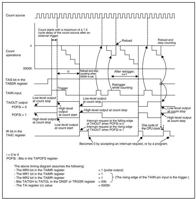
Figure 17.10 Operation Example in One-Shot Timer Mode
