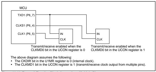
Figure 23.10 Transmit/Receive Clock Output from Multiple Pins
