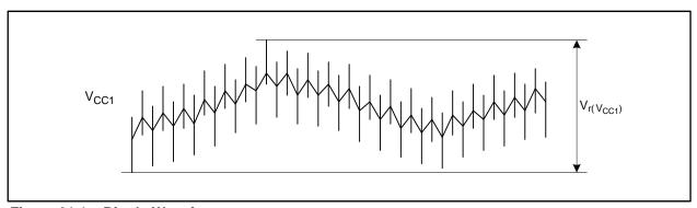
Figure 31.1 Ripple Waveform
