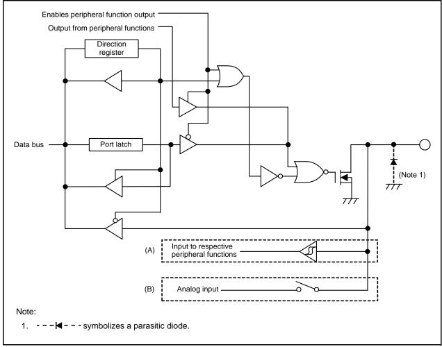
Figure 13.8 I/O Ports (N-channel Open Drain Output)
