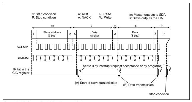
Figure 25.20 Example of Slave Transmission
