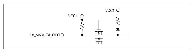
Figure 26.19 CEC External Circuit
