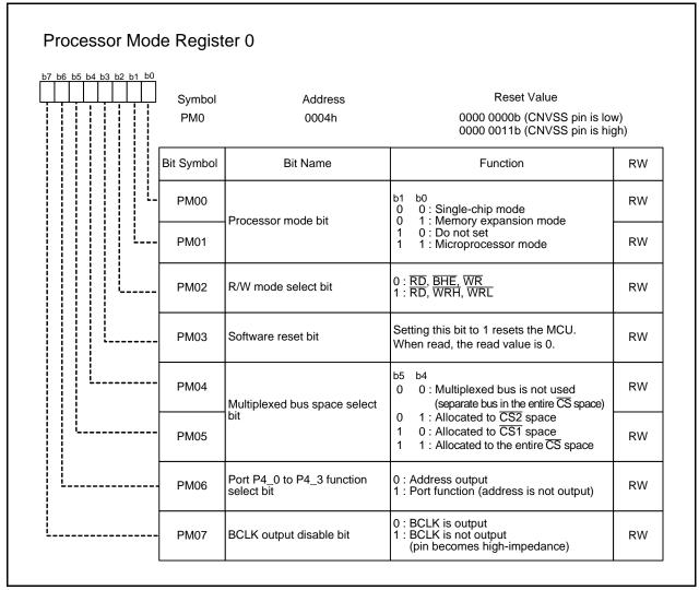
Set the PRC1 bit in the PRCR register to 1 (write enabled) before rewriting this register. Bits PM01 to PM00 do not change at software reset, watchdog timer reset, oscillator stop detect reset, voltage monitor 1 reset, or voltage monitor 2 reset.
