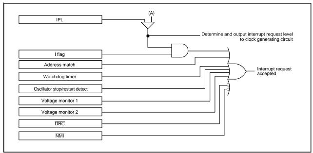
Figure 14.9 Interrupt Priority Select Circuit 2
