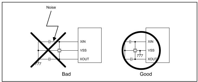
Figure 32.6 Clock I/O Pin Wiring
