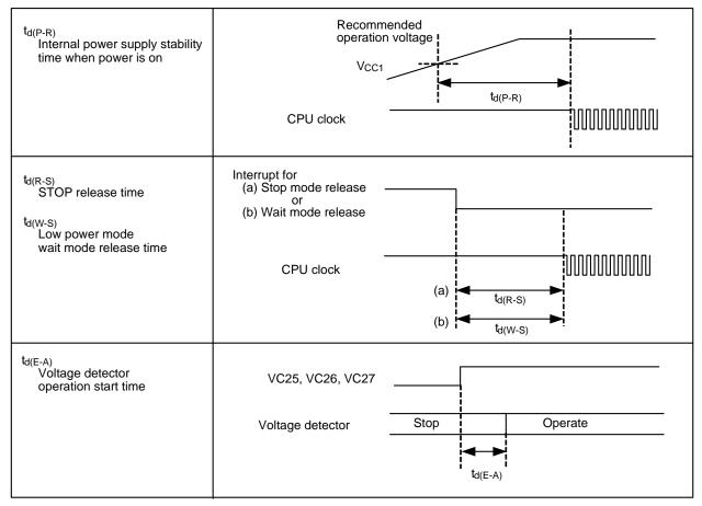
Figure 31.4 Power Supply Circuit Timing Diagram
