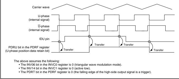
Figure 19.5 Position-Data-Retain Function (U-Phase) Operation
