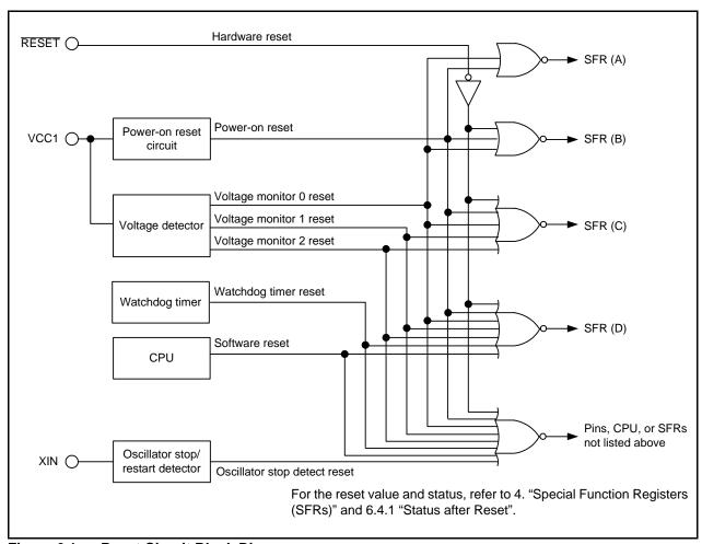
Figure 6.1 Reset Circuit Block Diagram
