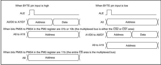
Figure 11.3 ALE Signal, Address Bus, and Data Bus
