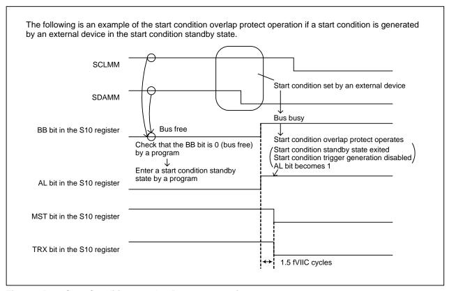
Figure 25.10 Start Condition Overlap Protect Operation
