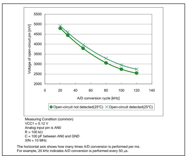
Figure 27.7 A/D Open-Circuit Detection (Charge) Characteristics (Standard Characteristics)
