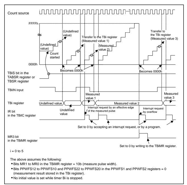
Figure 18.7 Operation Example in Pulse Width Measurement Mode
