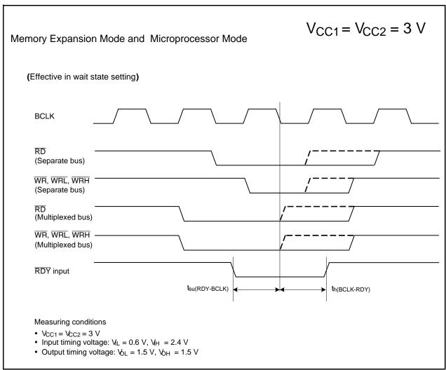
Figure 31.26 Timing Diagram
