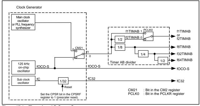
Figure 17.1 Timer A and B Count Sources
