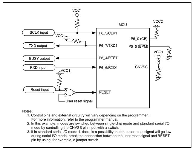
Figure 30.17 Circuit Application in Standard Serial I/O Mode 1
