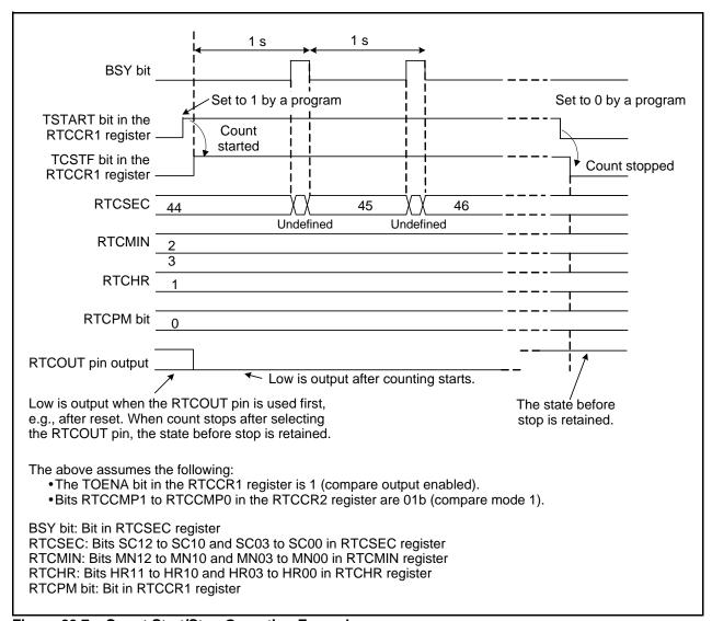
Figure 20.7 Count Start/Stop Operating Example
