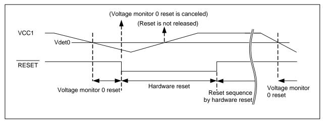
Figure 6.9 Hardware Reset when VCC1 < Vdet0
