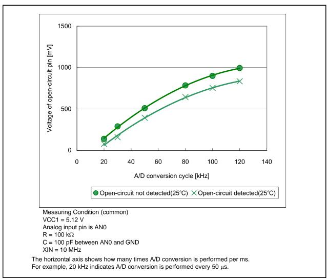
Figure 27.9 A/D Open-Circuit Detection (Discharge) Characteristics (Standard Characteristics)
