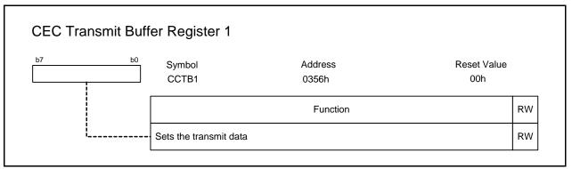
Rewrite the CCTB1 register when the CTXDEN bit in the CECC3 register is 0 (transmit disabled), or the CTXDEN bit is 1 and the CTD8FLG in the CECFLG register is 1 (while bits EOM and ACK are being transmitted after the eighth bit has been transmitted). Do not rewrite the CCTB1 register when the CTXDEN bit is 1 and the CTD8FLG bit is 0 (while the first bit to eighth bit are being transmitted).
