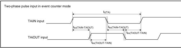
Figure 31.21 Timer A Input (Two-Phase Pulse Input in Event Counter Mode)
