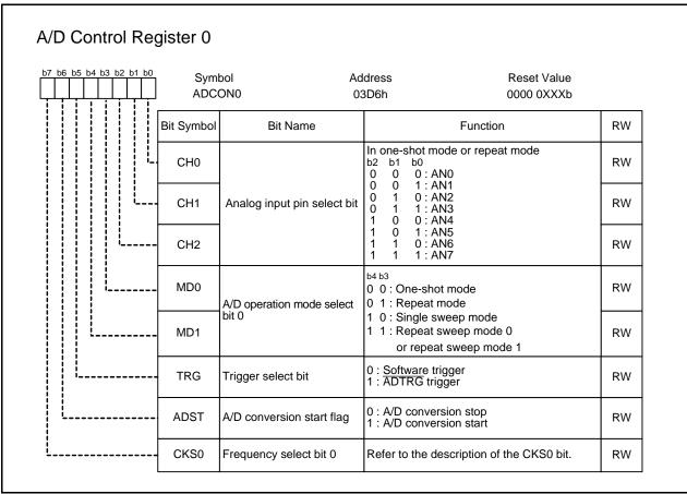
If the ADCON0 register is rewritten during A/D conversion, the conversion result is undefined.
