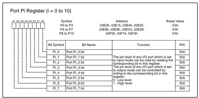
Data input/output to and from external devices is accomplished by reading and writing to the Pi register. Each bit in the Pi register consists of a port latch to hold the output data and a circuit to read the pin status.
