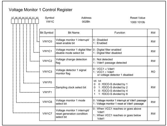
Set the PRC3 bit in the PRCR register to 1 (write enabled) before rewriting this register.
