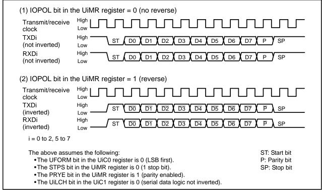
Figure 23.16 TXD and RXD I/O Polarity Inversion
