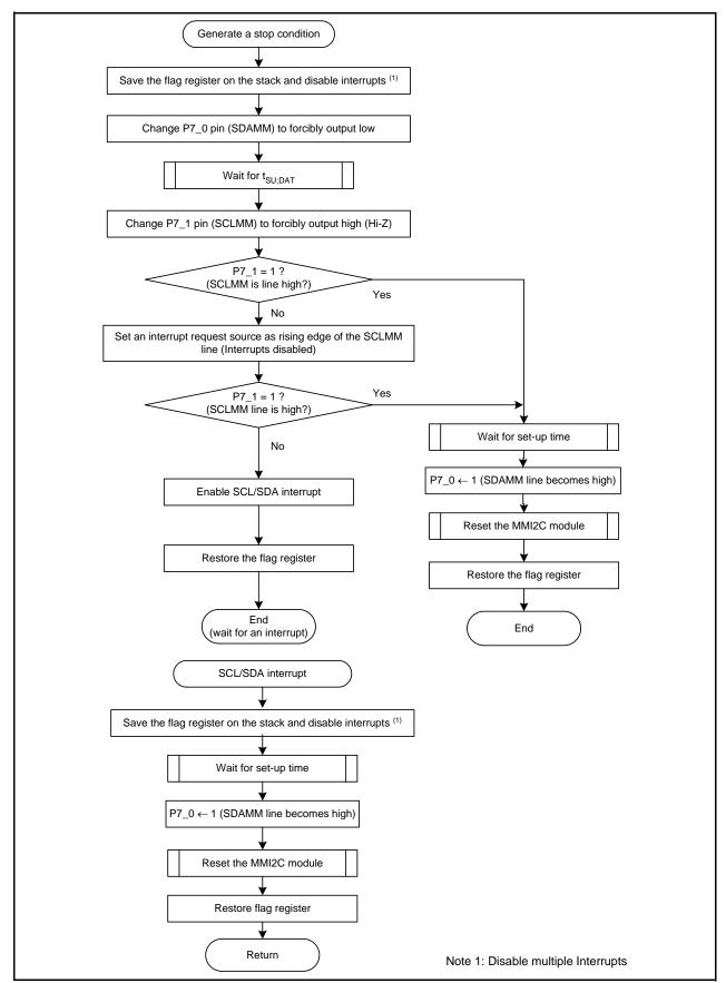
Figure 25.23 Generating a Stop Condition
