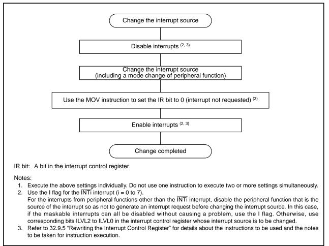
Figure 32.10 Procedure for Changing the Interrupt Generate Source
