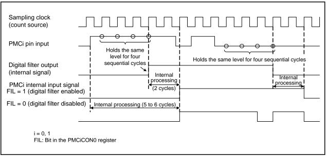
Figure 22.5 PMCi Input Delay
