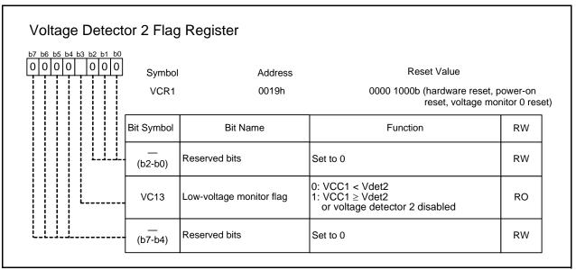
This register does not change at voltage monitor 1 reset, voltage monitor 2 reset, oscillator stop detect reset, watchdog timer reset, or software reset.
