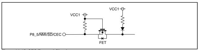
Figure 32.15 CEC External Circuit
