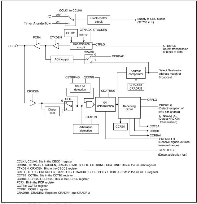
Figure 26.1 CEC Function Block Diagram
