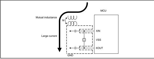
Figure 32.7 Large Current Signal Line Wiring
