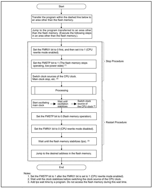
Figure 9.3 Stop and Restart of the Flash Memory
