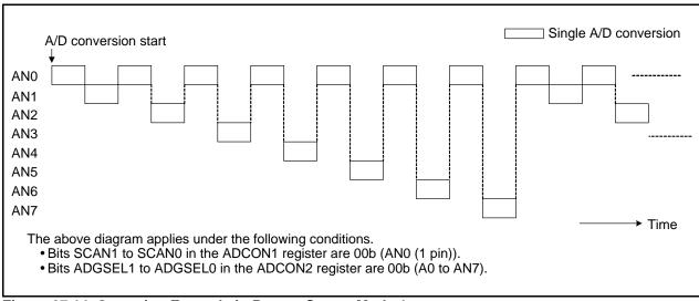
Figure 27.14 Operation Example in Repeat Sweep Mode 1
