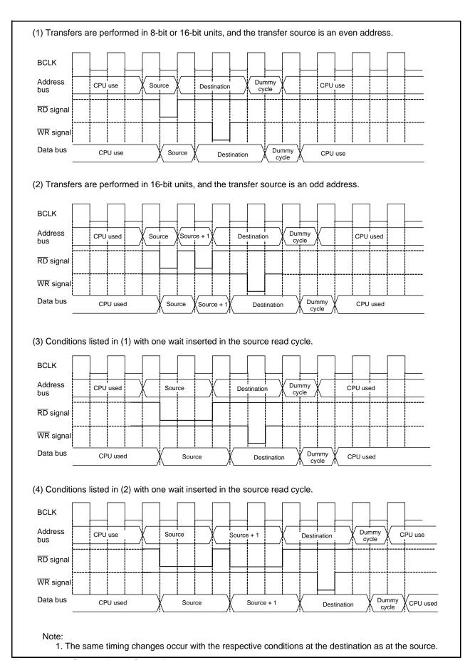
Figure 16.2 Source Read Cycle Example
