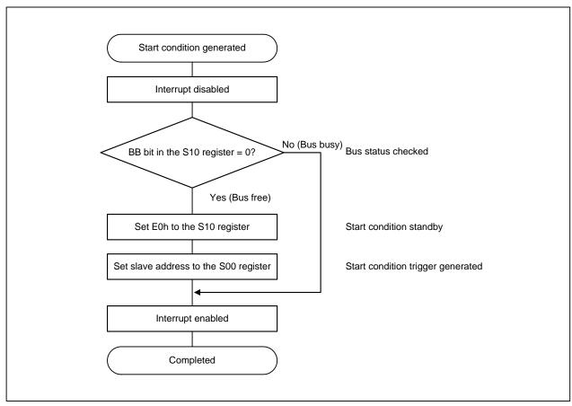
Figure 25.6 Procedure to Generate a Start Condition
