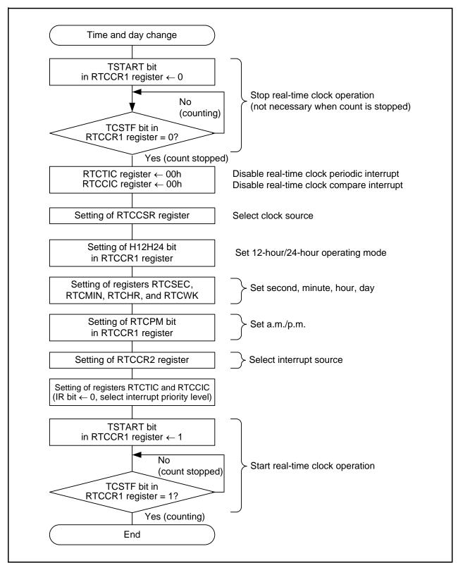
Figure 20.4 Time and Day Change Procedure (No Compare Mode or Compare Mode 1)
