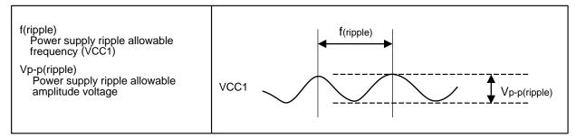
Figure 8.11 Voltage Fluctuation Timing
