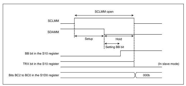
Figure 25.13 Start Condition Detection
