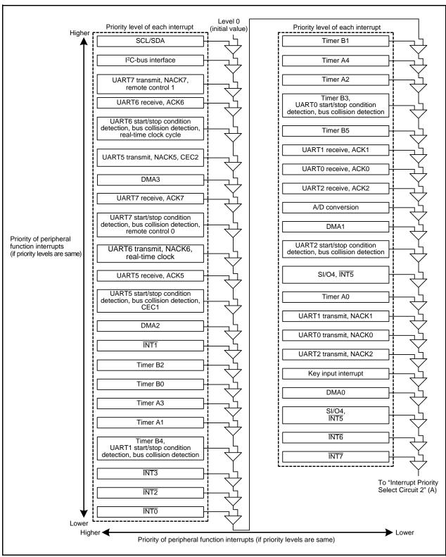
Figure 14.8 Interrupt Priority Select Circuit 1
