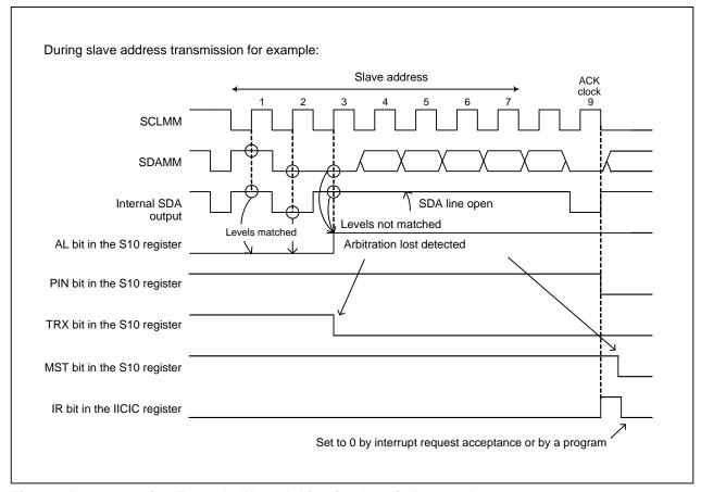
Figure 25.12 Operation Example When Arbitration Lost is Detected
