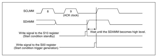
Figure 25.9 Restart Condition Generation Timing
