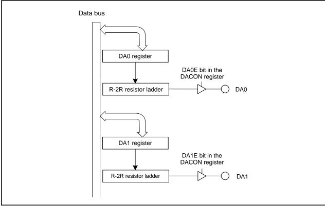
Figure 28.1 D/A Converter Block Diagram
