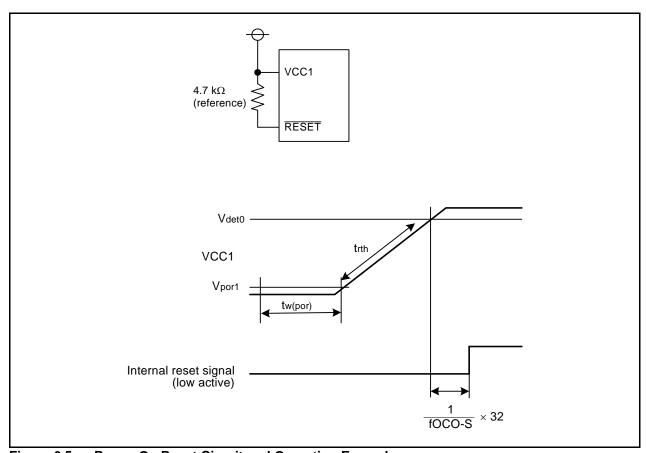
Figure 6.5 Power-On Reset Circuit and Operation Example
