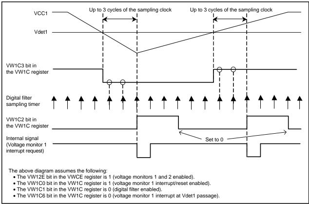
Figure 7.2 Digital Filter Operation Example
