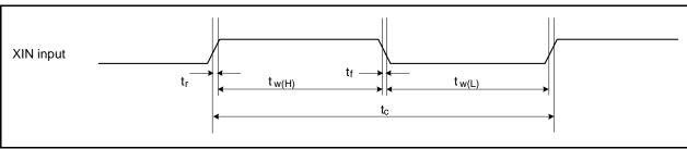
Figure 31.19 External Clock Input (XIN Input)
