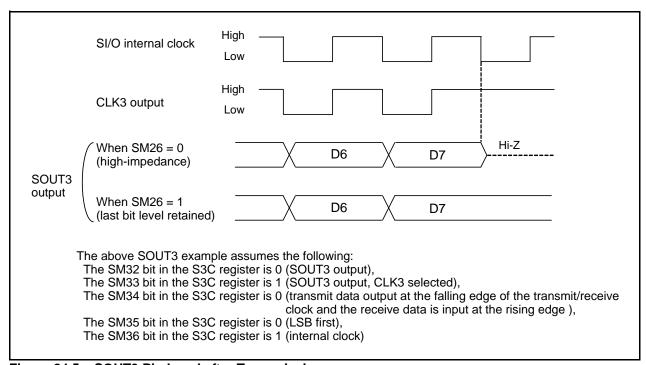
Figure 24.5 SOUT3 Pin Level after Transmission
