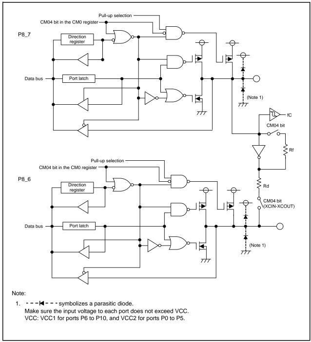
Figure 13.10 I/O Ports (XC)
