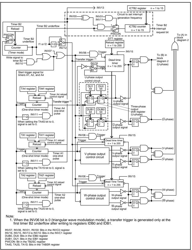
Figure 19.1 Three-Phase Motor Control Timer Function Block Diagram 1
