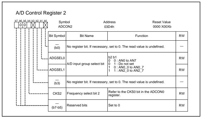
If the ADCON2 register is rewritten during A/D conversion, the conversion result is undefined.
