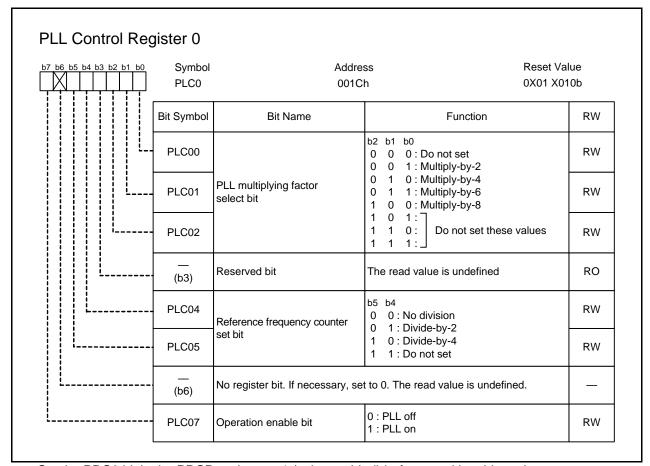
Set the PRC0 bit in the PRCR register to 1 (write enabled) before rewriting this register.
