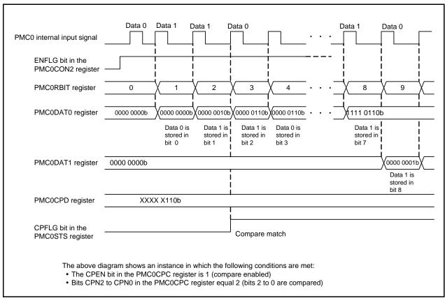
Figure 22.8 Receive Buffer and Compare Function
