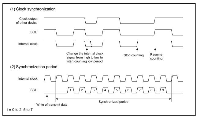
Figure 23.25 Clock Synchronization
