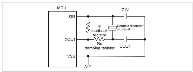
Figure 32.5 Oscillator Example
