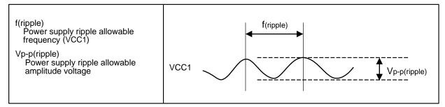
Figure 32.9 Voltage Fluctuation Timing
