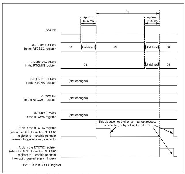
Figure 20.3 Real-Time Clock Basic Operating Example
