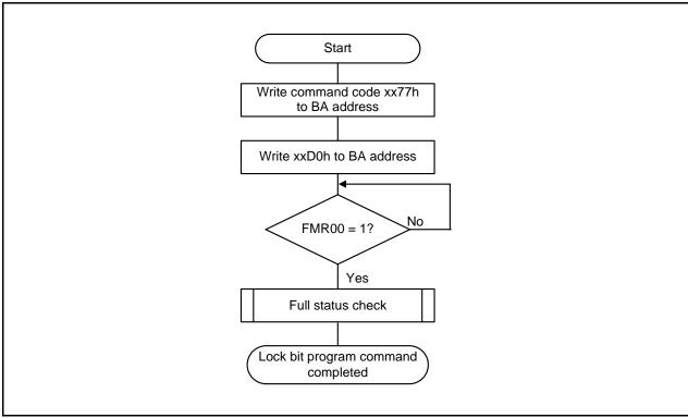
Figure 30.12 Lock Bit Program Command
