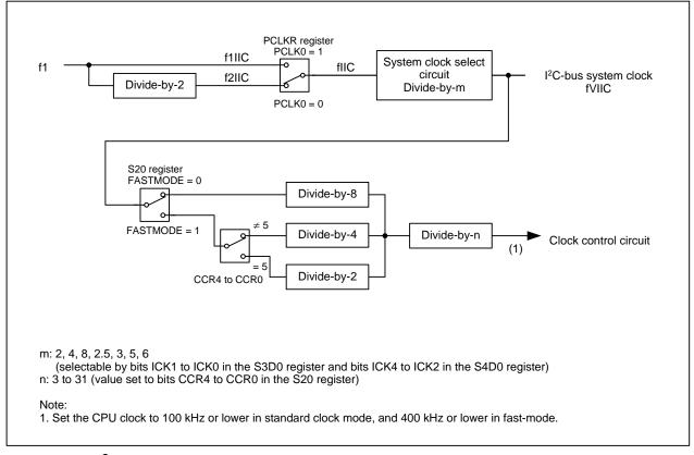
Figure 25.5 I<sup>2</sup>C-bus Interface Clock
