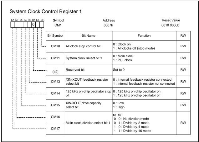
Rewrite the CM1 register after setting the PRC0 bit in the PRCR register to 1 (write enabled). See Table 9.3 "Clock-Related Bit Setting and Modes" to select a clock and a mode.
