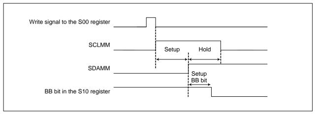
Figure 25.8 Stop Condition Generation Timing
