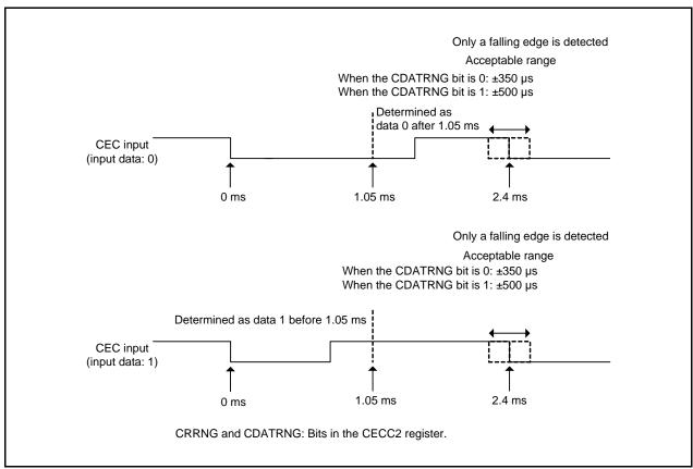
Figure 26.6 Data Bit Acceptable Range (CRRNG Bit = 0)
