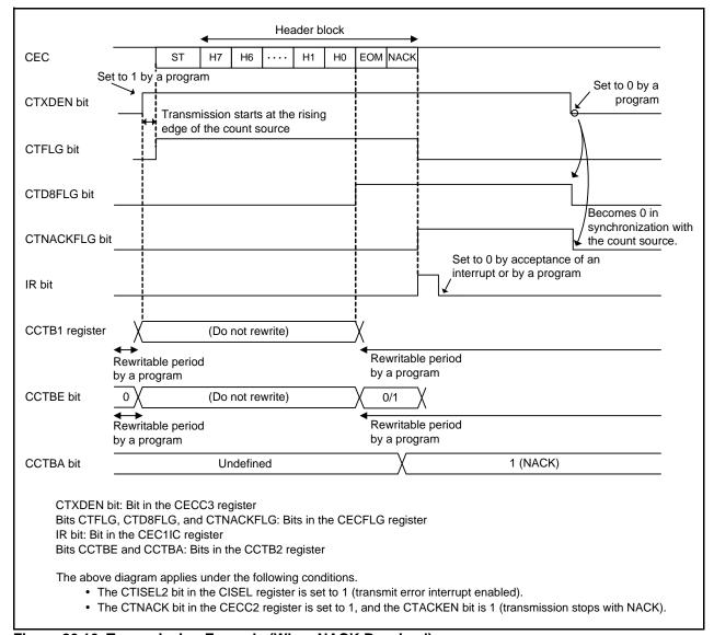
Figure 26.16 Transmission Example (When NACK Received)
