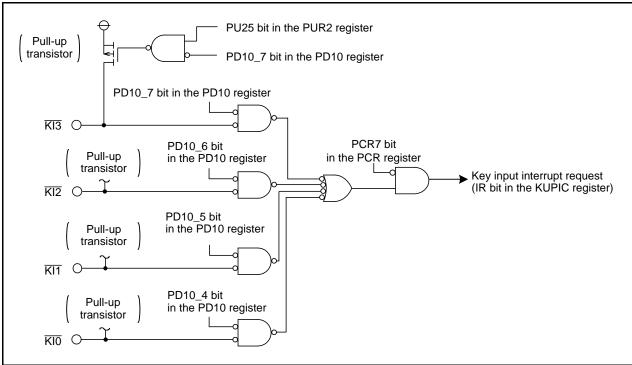
Figure 14.11 Block Diagram of Key Input Interrupt
