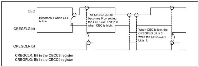
Figure 26.2 Operation of Bits CREGFLG and CREGCLR
