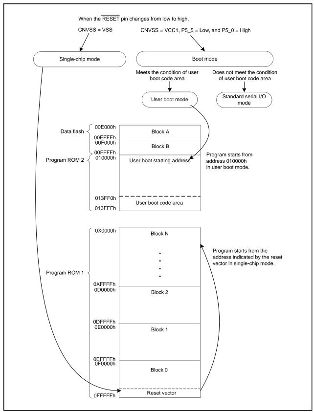
Figure 30.4 Program Starting Address in User Boot Mode
