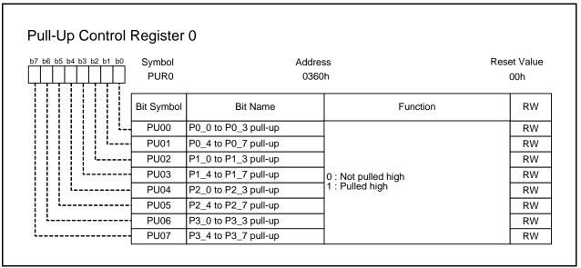
In memory expansion or microprocessor mode, the register value can be modified, but the pins are not pulled high.
