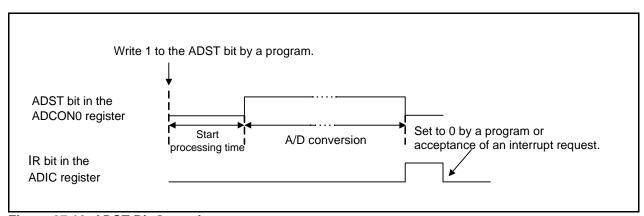
Figure 27.18 ADST Bit Operation
