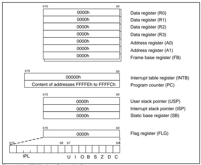
Figure 6.2 CPU Register Status after Reset
