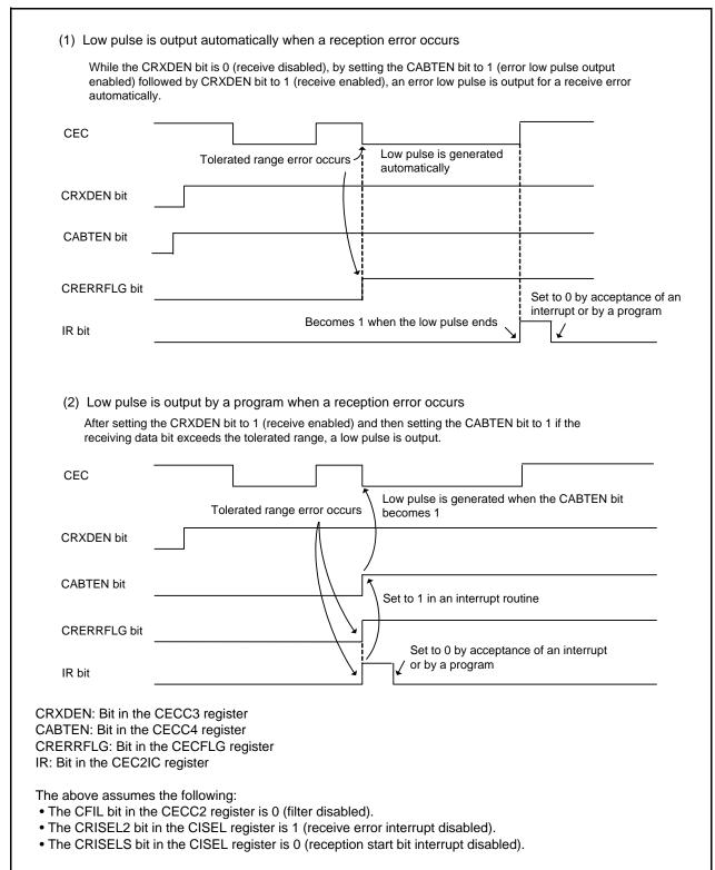
Figure 26.9 Low Pulse Output Timing in Receive Error
