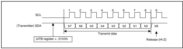
Figure 23.28 Byte Data Transmission
