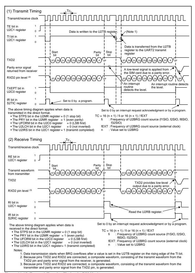
Figure 23.35 Transmit/Receive Timing in SIM Mode
