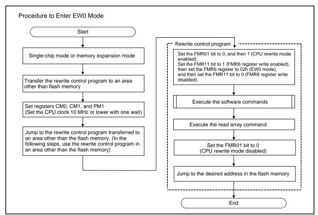
Figure 30.5 Setting and Resetting of EW0 Mode
