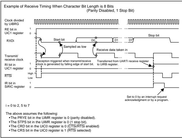
Figure 23.13 Receive Timing in UART Mode
