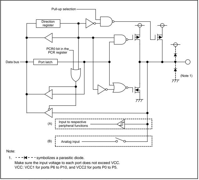
Figure 13.3 I/O Ports (Port P1)
