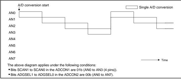
Figure 27.13 Operation Example in Repeat Sweep Mode 0
