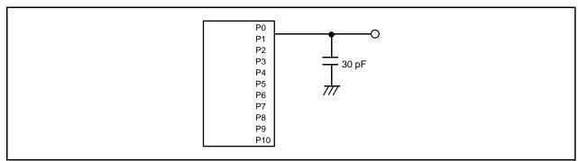
Figure 31.27 Ports P0 to P10 Measurement Circuit
