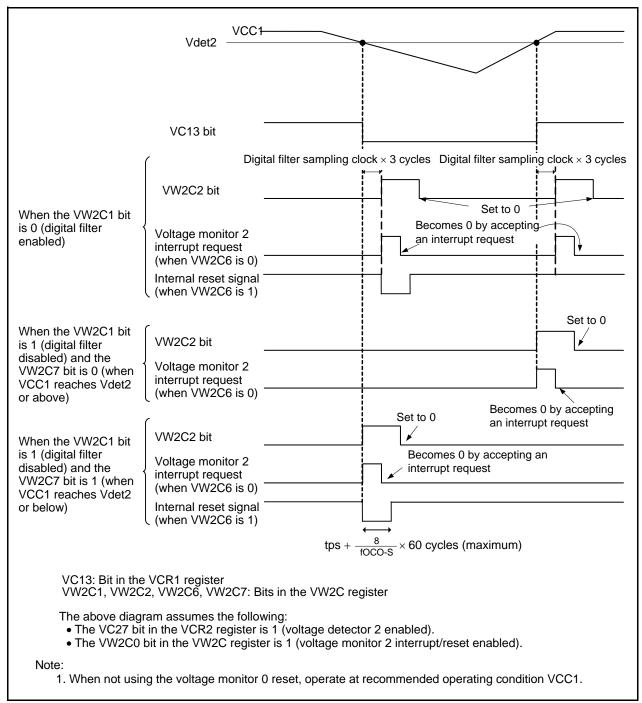
Figure 7.8 Voltage Monitor 2 Interrupt/Reset Operation Example
