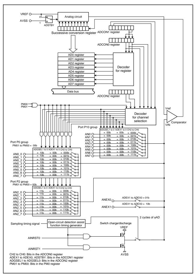
Figure 27.1 A/D Converter Block Diagram
