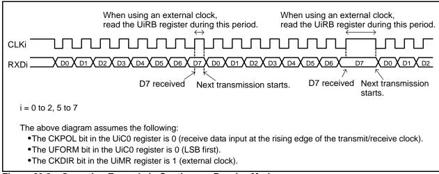
Figure 23.8 Operation Example in Continuous Receive Mode
