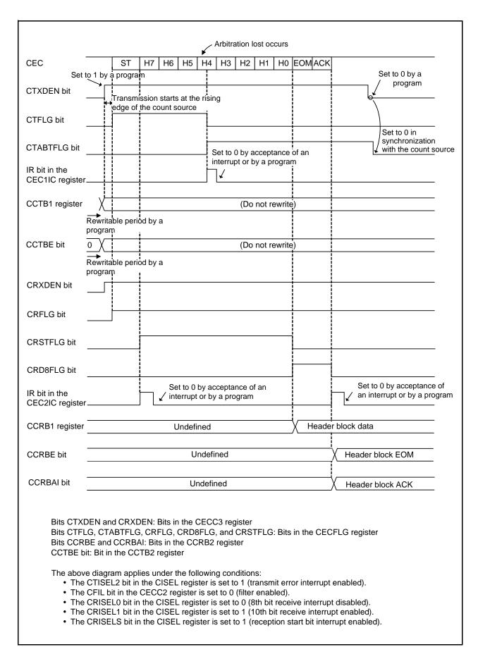
Figure 26.17 Transmission Example (When an Arbitration Lost Detected)
