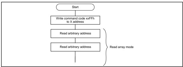
Figure 30.7 Read Array Command
