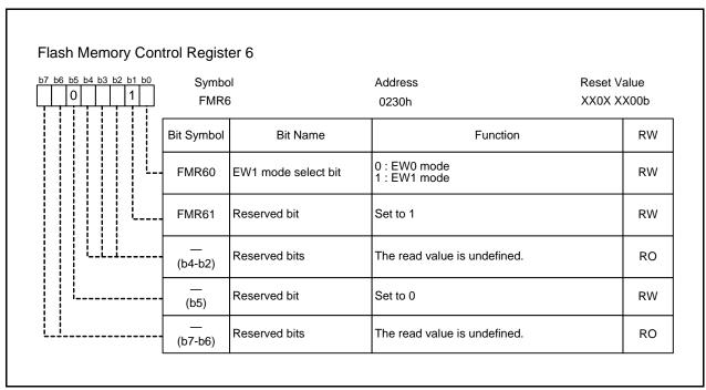
When accessing the FMR6 register, select a CPU clock frequency of 10 MHz or less by setting the CM06 bit in the CM0 register and bits CM17 and CM16 in the CM1 register. Also, set the PM17 bit in the PM1 register to 1 (wait state).
