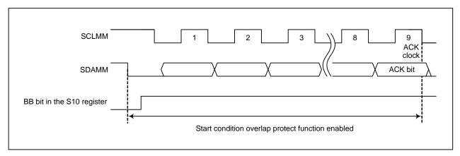
Figure 25.11 Start Condition Overlap Protect Function Enable Period
