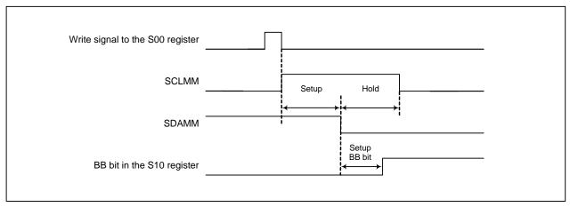
Figure 25.7 Start Condition Generation Timing
