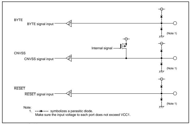
Figure 13.12 I/O Pins
