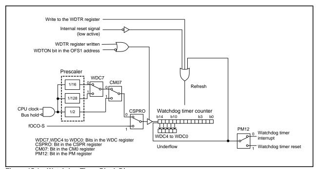
Figure 15.1 Watchdog Timer Block Diagram
