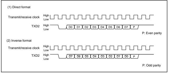
Figure 23.38 SIM Interface Format
