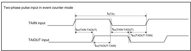
Figure 31.8 Timer A Input (Two-Phase Pulse Input in Event Counter Mode)
