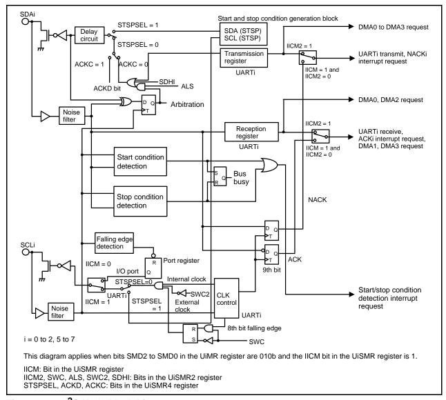
Figure 23.18 I<sup>2</sup>C Mode Block Diagram
