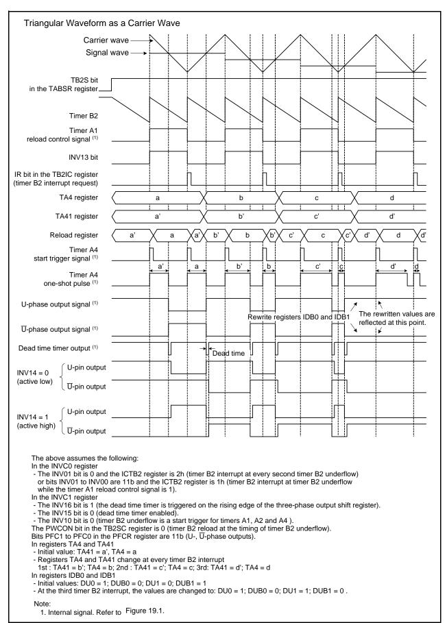
Figure 19.7 Example of Three-Phase Mode 1 Operation
