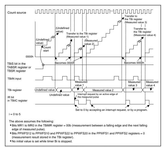
Figure 18.6 Operation Example in Pulse Period Measurement Mode
