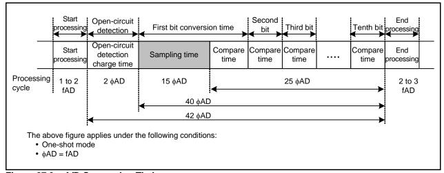
Figure 27.3 A/D Conversion Timing
