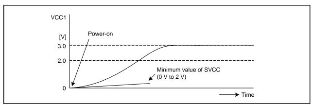
Figure 6.8 SVCC Timing (VCC1 ≤ 3.6 V)
