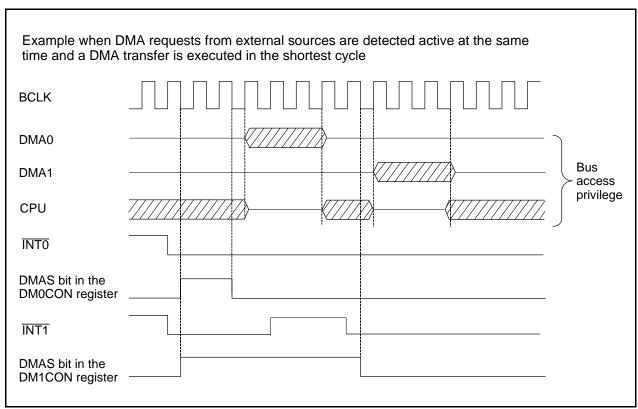
Figure 16.5 DMA Transfer Initiated by External Sources
