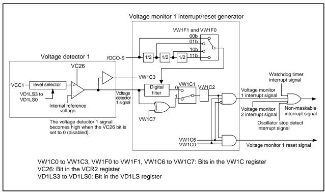
Figure 7.5 Voltage Monitor 1 Interrupt/Reset Generator
