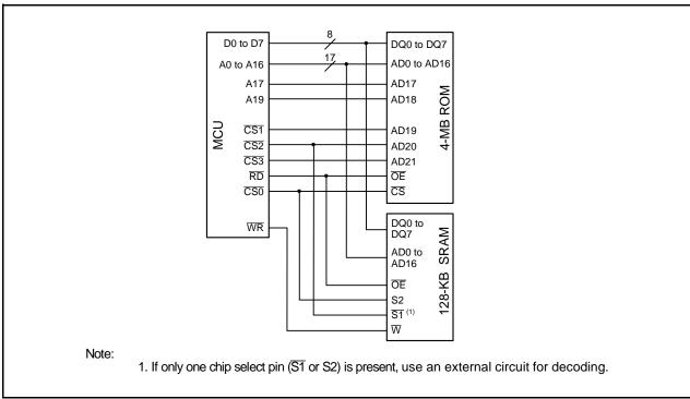
Figure 12.5 External Memory Connection Example in 4-MB Mode
