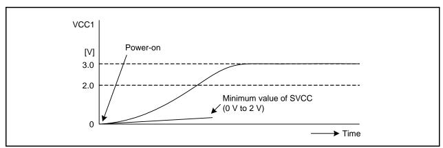
Figure 32.3 SVCC Timing (VCC1 ≤ 3.6 V)
