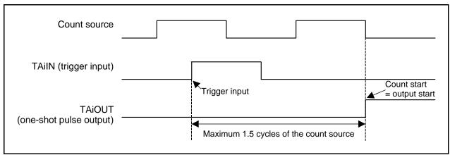
Figure 17.4 Output Example of One-Shot Timer Mode
