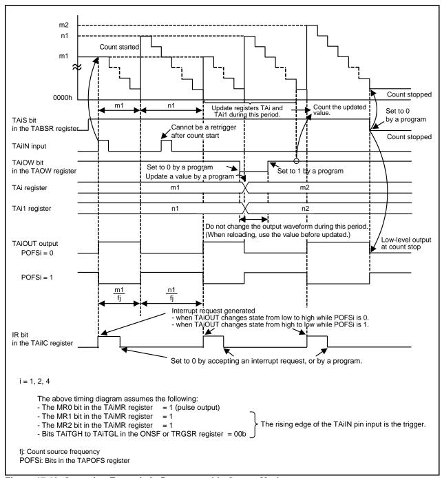
Figure 17.13 Operation Example in Programmable Output Mode
