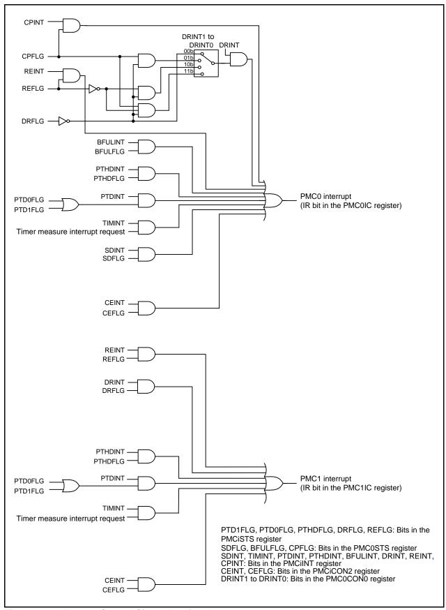
Figure 22.10 Remote Control Signal Receiver Interrupts
