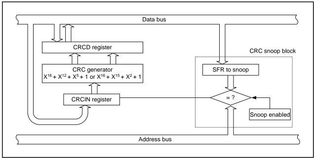
Figure 29.1 CRC Calculator Block Diagram
