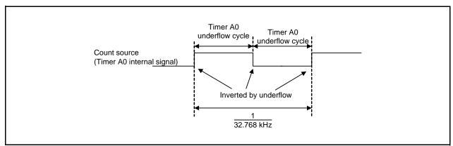
Figure 26.3 Count Source When Timer A0 Underflow Selected
