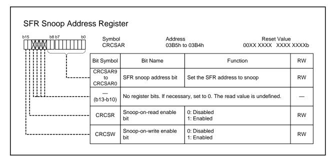
CRCSR (Snoop-on-read enable bit) (b14) CRCSW (Snoop-on-write enable bit) (b15)
