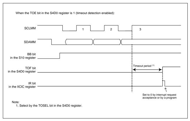
Figure 25.16 Timeout Detection Timing
