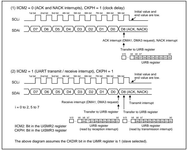
Figure 23.20 Transfer to UiRB Register and Interrupt Timing
