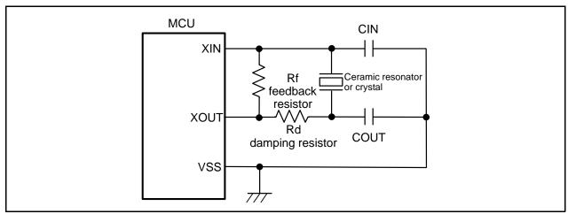
Figure 8.7 Oscillator Example
