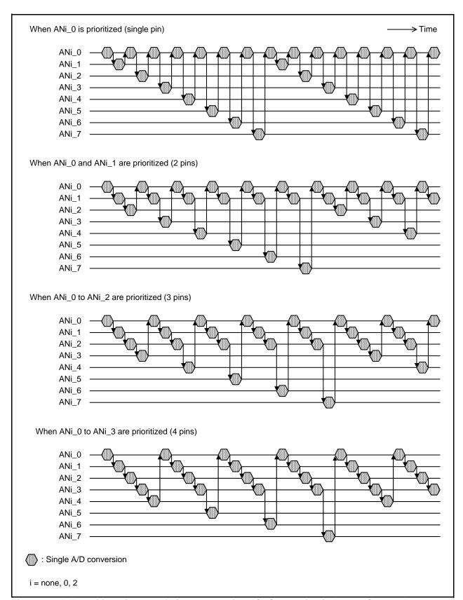
Figure 27.15 Transition Diagram of Pins Used during A/D Conversion in Repeat Sweep Mode 1
