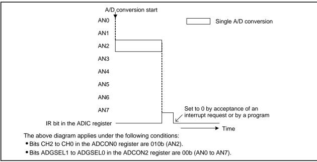
Figure 27.10 Operation Example in One-Shot Mode
