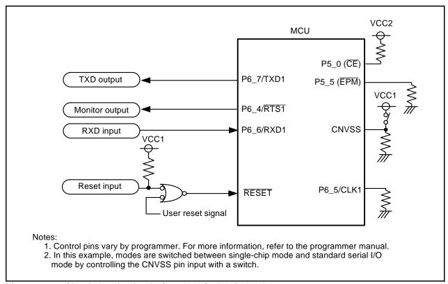
Figure 30.18 Circuit Application in Standard Serial I/O Mode 2
