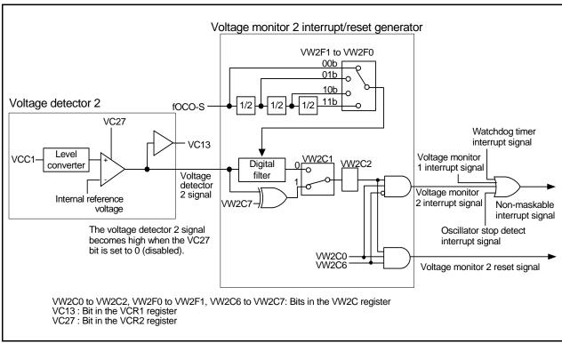
Figure 7.7 Voltage Monitor 2 Interrupt/Reset Generator
