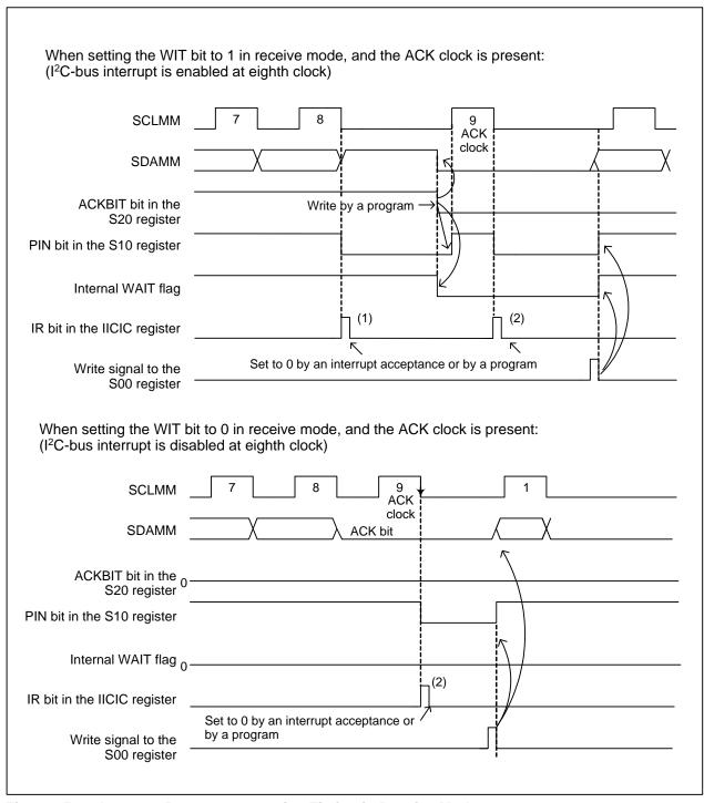
Figure 25.4 Interrupt Request Generation Timing in Receive Mode
