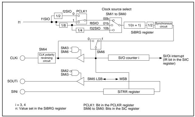
Figure 24.1 SI/O3 and SI/O4 Block Diagram
