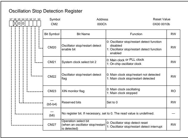
Set the PRC0 bit in the PRCR register to 1 (write enabled) before rewriting this register.
