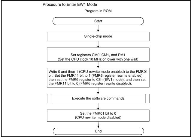
Figure 30.6 Setting and Resetting of EW1 Mode
