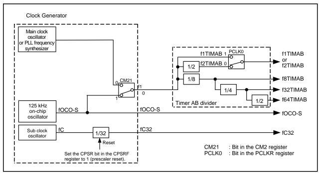
Figure 18.1 Timer A and B Count Sources
