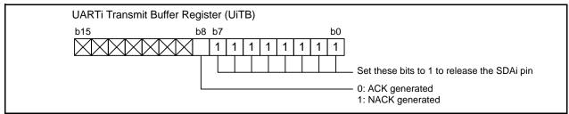
Figure 23.30 UiTB Register Setting (SDA Input)
