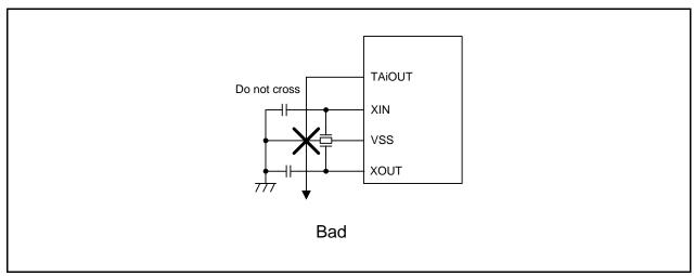
Figure 8.10 Wiring of Signal Line Whose Level Changes at High-Speed
