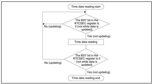
Figure 32.11 Time Data Reading
