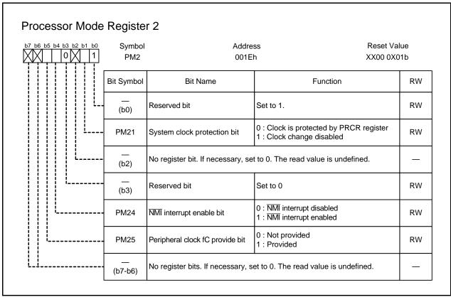
Set the PRC1 bit in the PRCR register to 1 (write enabled) before rewriting this register.
