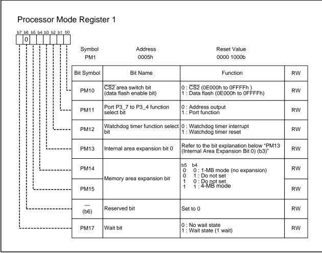
Set the PRC1 bit in the PRCR register to 1 (write enabled) before rewriting this register.
