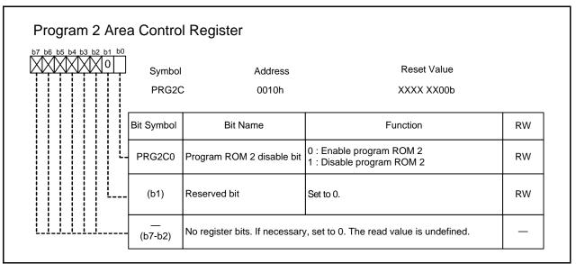
Set the PRC6 bit in the PRCR register to 1 (write enabled) before rewriting this register.
