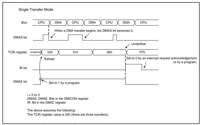
Figure 16.3 Operation Example in Single Transfer Mode
