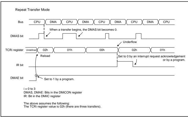
Figure 16.4 Operation Example in Repeat Transfer Mode
