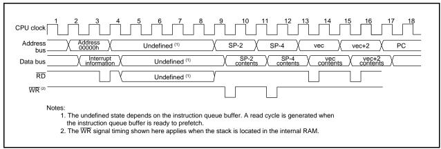
Figure 14.3 Time Required for Executing Interrupt Sequence
