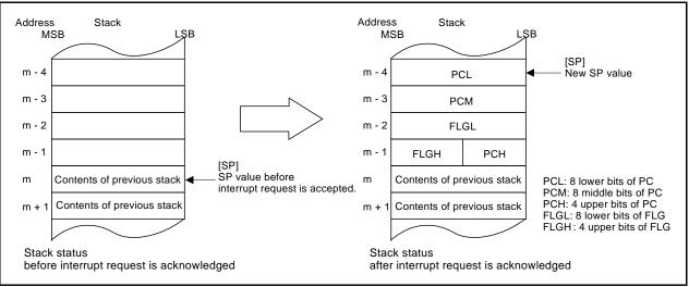
Figure 14.5 Stack Status Before and After Acceptance of Interrupt Request
