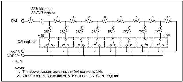
Figure 28.2 D/A Converter Equivalent Circuit
