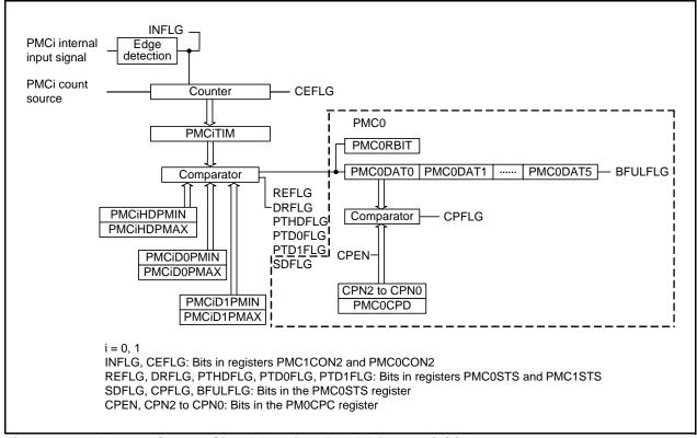
Figure 22.1 Remote Control Signal Receiver Block Diagram (1/3)
