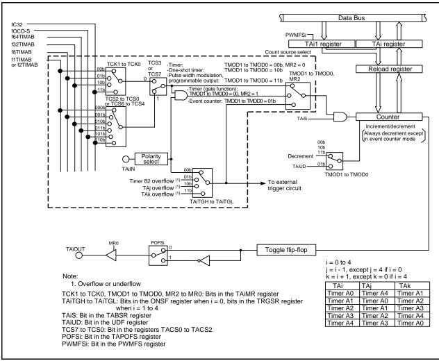
Figure 17.3 Timer A Block Diagram
