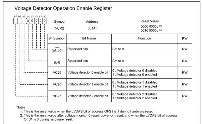
Set the PRC3 bit in the PRCR register to 1 (write enabled) before rewriting this register.
