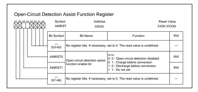
AINRST1-AINRST0 (Open-circuit detection assist function enable bit) (b5-b4)
