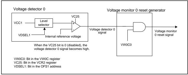
Figure 7.3 Voltage Monitor 0 Reset Generator Block Diagram
