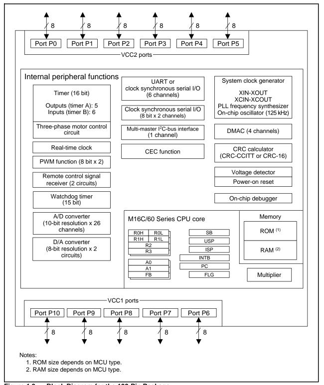
Figure 1.3 Block Diagram for the 100-Pin Package
