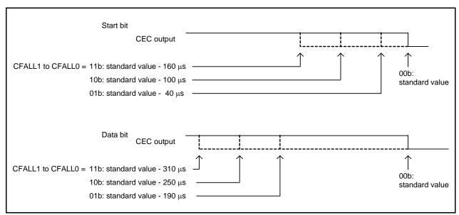
Figure 26.13 Falling Timing of Transmit Signal
