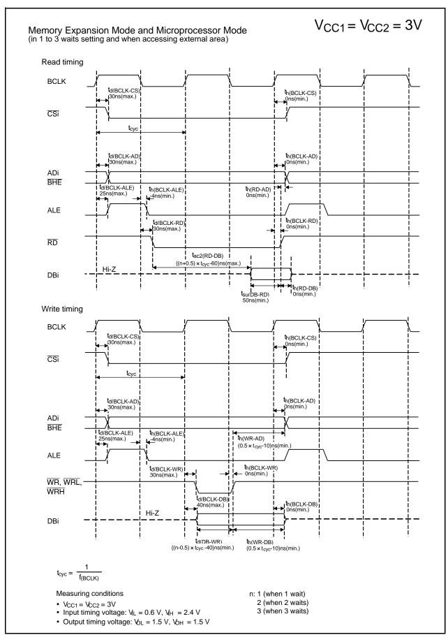
Figure 31.29 Timing Diagram
