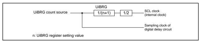
Figure 23.19 Internal Clock Configuration
