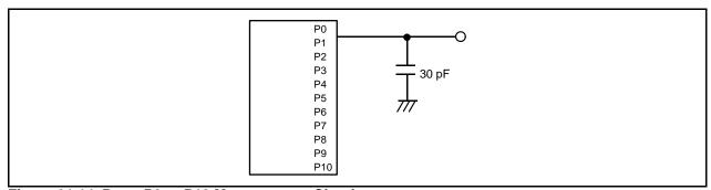
Figure 31.14 Ports P0 to P10 Measurement Circuit
