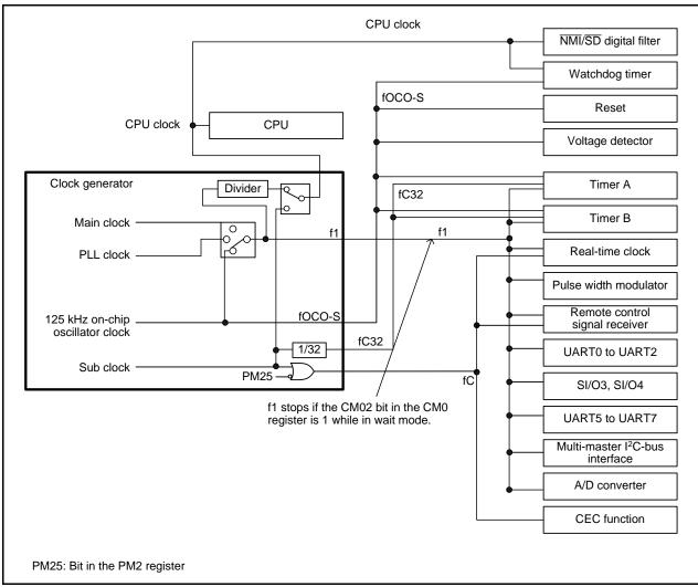
Figure 8.5 Peripheral Function Clocks
