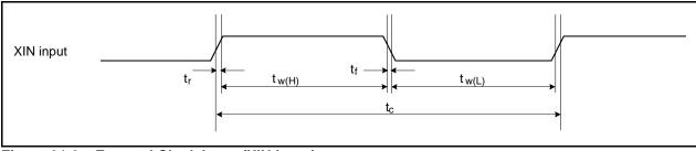
Figure 31.6 External Clock Input (XIN Input)
