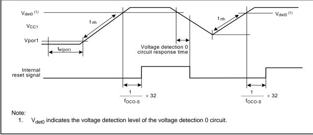
Figure 31.3 Power-On Reset Circuit Electrical Characteristics
