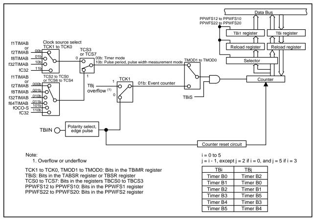
Figure 18.3 Timer B Block Diagram
