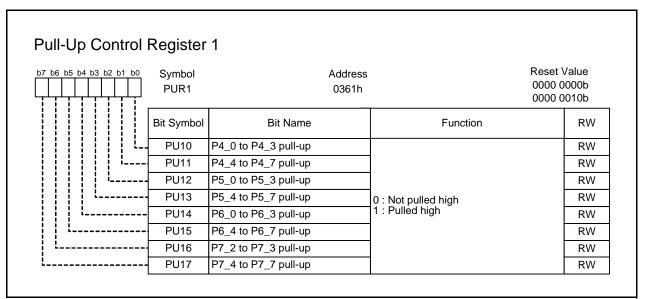
Values after hardware reset, power-on reset, or voltage monitor 0 reset are as follows:
