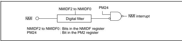
Figure 14.10 NMI Interrupt Block Diagram
