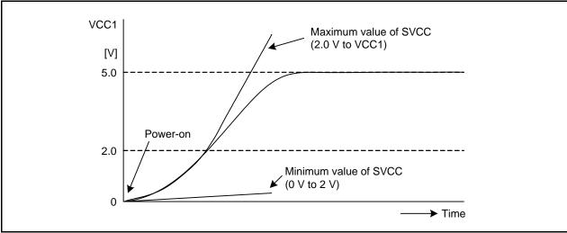
Figure 6.7 SVCC Timing (3.6 V < VCC1)
