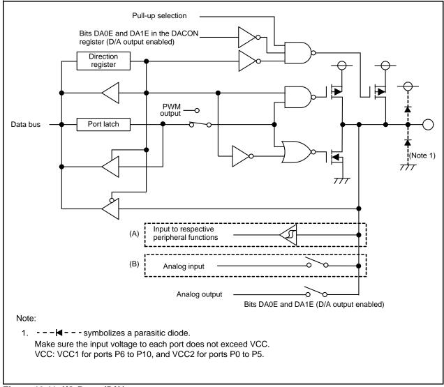
Figure 13.11 I/O Ports (D/A)
