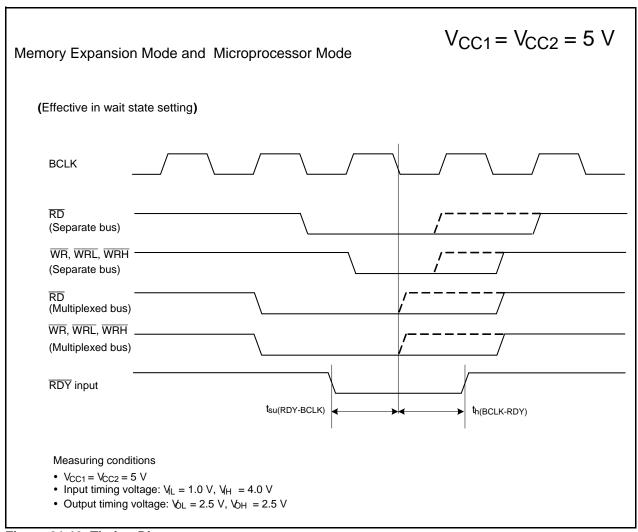
Figure 31.13 Timing Diagram
