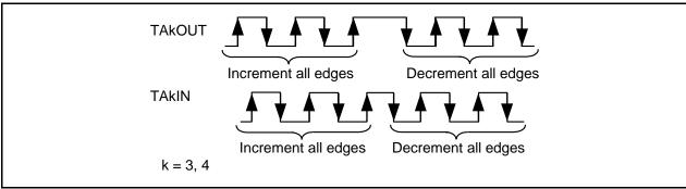
Figure 17.8 Multiply-by-4 Processing
