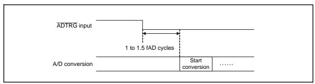
Figure 27.5 A/D Conversion Start Timing When External Trigger Input
