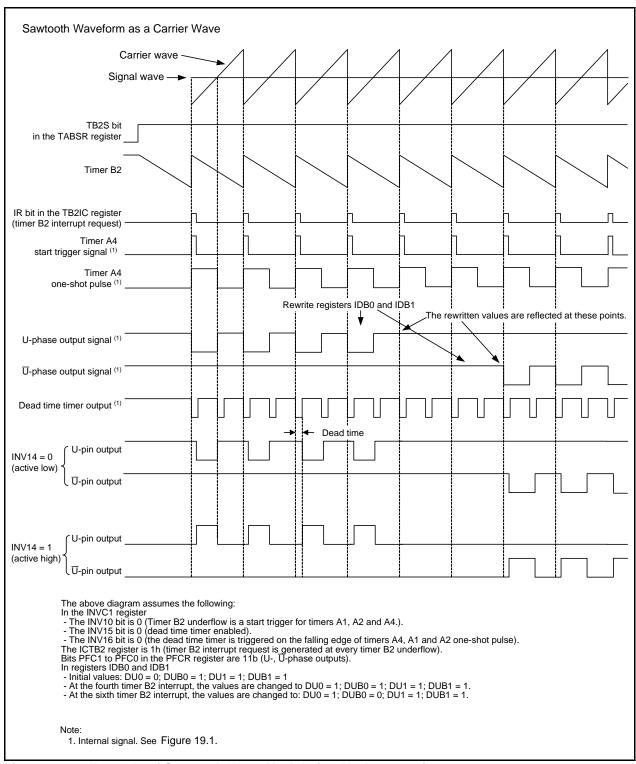
Figure 19.9 Example of Sawtooth Wave Modulation Mode Operation
