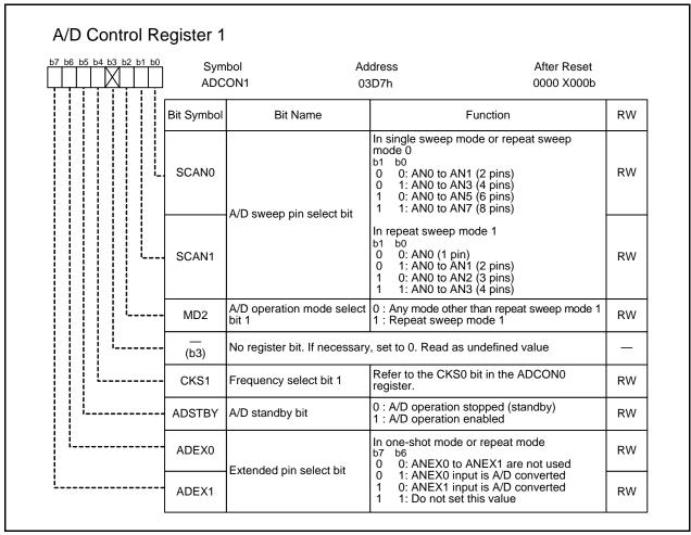
If the ADCON1 register is rewritten during A/D conversion, the conversion result is undefined.
