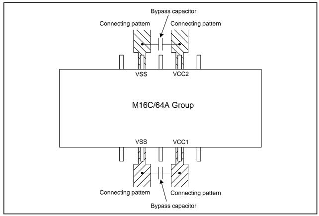
Figure 32.1 Bypass Capacitor Connection
