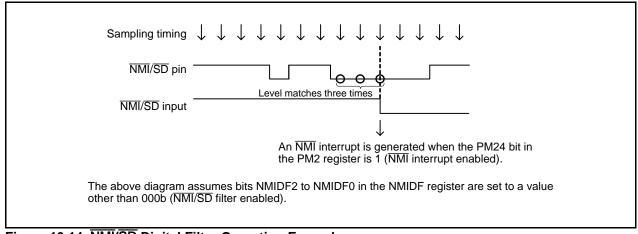
Figure 13.14 NMI/SD Digital Filter Operation Example
