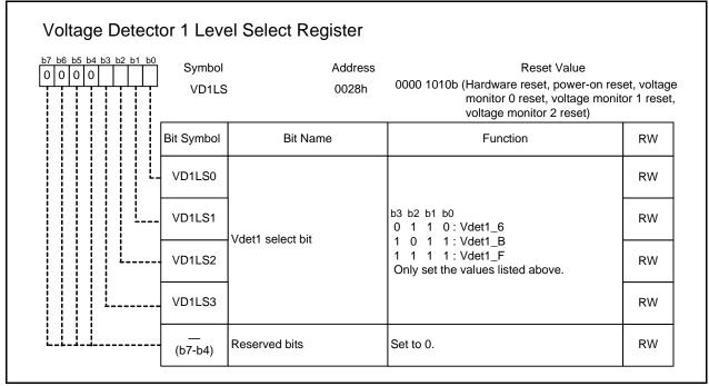
Set the PRC3 bit in the PRCR register to 1 (write enabled) before rewriting this register. Also, rewrite this register when the VW12E bit in the VWCE register is 1.
