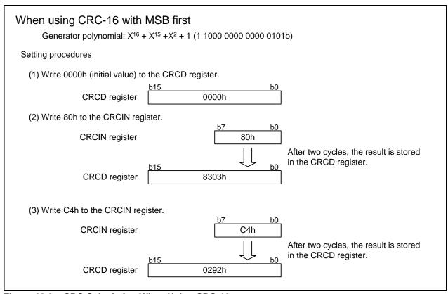
Figure 29.3 CRC Calculation When Using CRC-16
