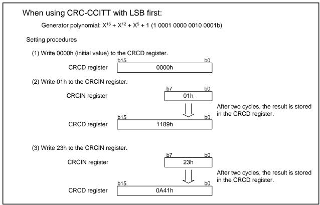
Figure 29.2 CRC Calculation When Using CRC-CCITT
