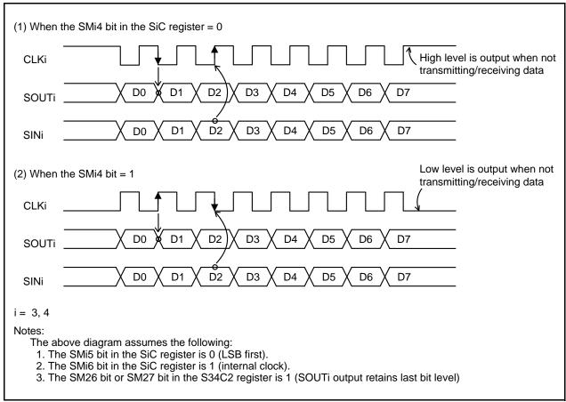
Figure 24.2 Polarity of Transmit/Receive Clock
