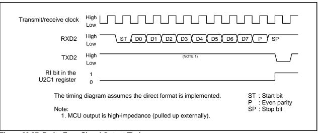
Figure 23.37 Parity Error Signal Output Timing
