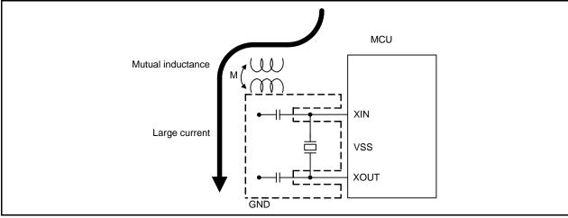
Figure 8.9 Large Current Signal Line Wiring
