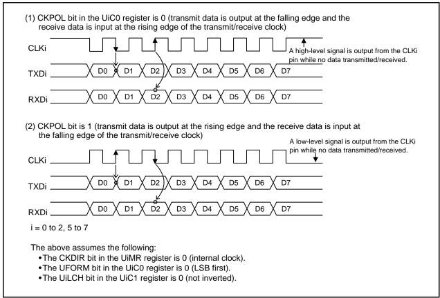
Figure 23.6 Transmit/Receive Clock Polarity
