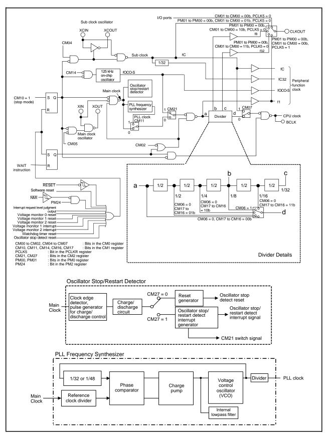
Figure 8.1 System Clock Generator
