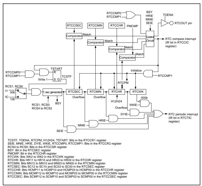
Figure 20.1 Real-Time Clock Block Diagram
