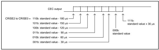
Figure 26.12 Rising Timing of Transmit Signal
