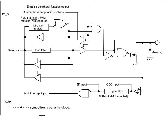
Figure 13.9 I/O Ports (NMI)
