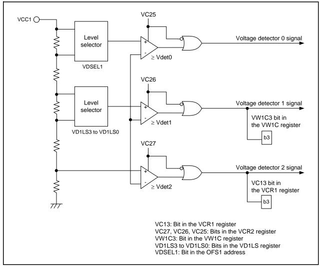
Figure 7.1 Voltage Detector Block Diagram
