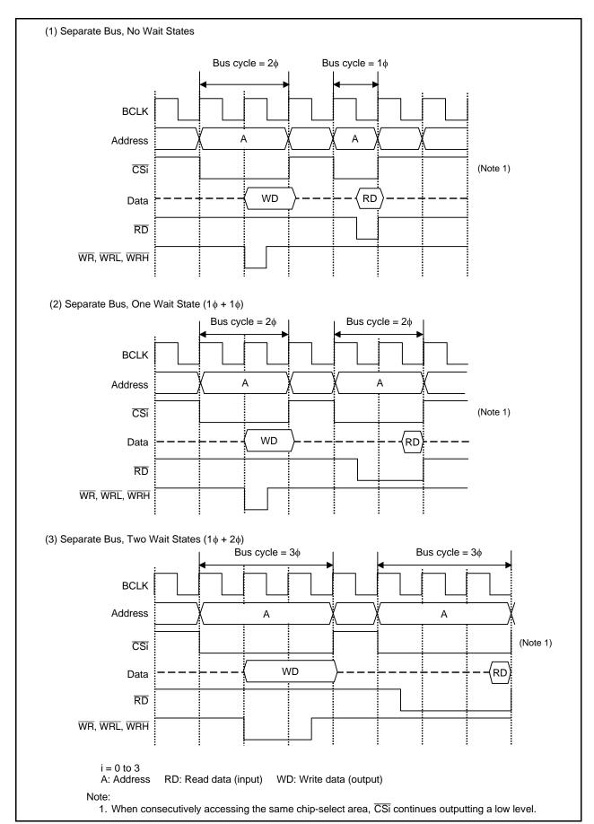
Figure 11.6 Typical Bus Timings Using Software Wait States (1/2)
