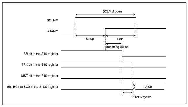
Figure 25.14 Stop Condition Detection
