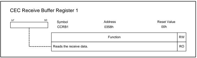
Read the CCRB1 register after receiving the eighth bit (the CRD8FLG bit in the CECFLG register changes from 0 to 1).
