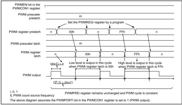
Figure 21.3 PWMi Output Example (Duty 0%, Duty 100%)
