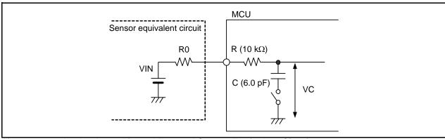
Figure 27.16 Analog Input Pin and External Sensor Equivalent Circuit
