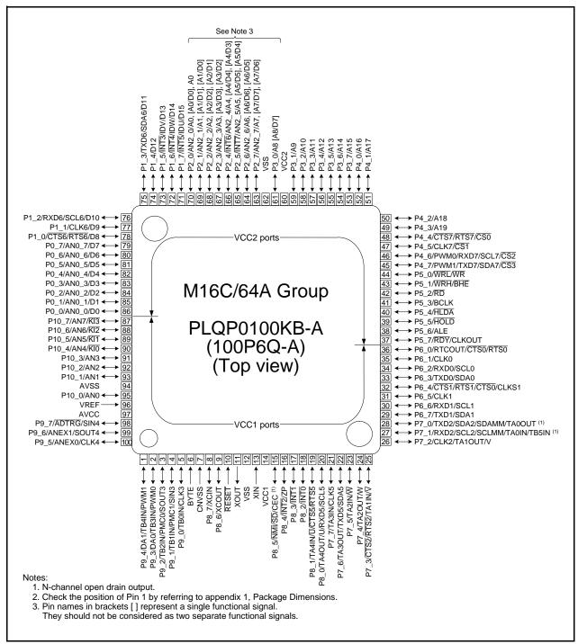
Figure 1.5 Pin Assignment for the 100-Pin Package
