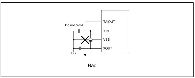
Figure 32.8 Wiring of Signal Line Whose Level Changes at High-Speed
