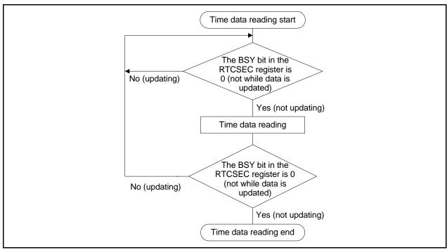
Figure 20.11 Time Data Reading
