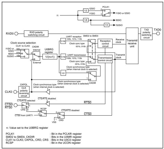
Figure 23.1 UARTO Block Diagram
