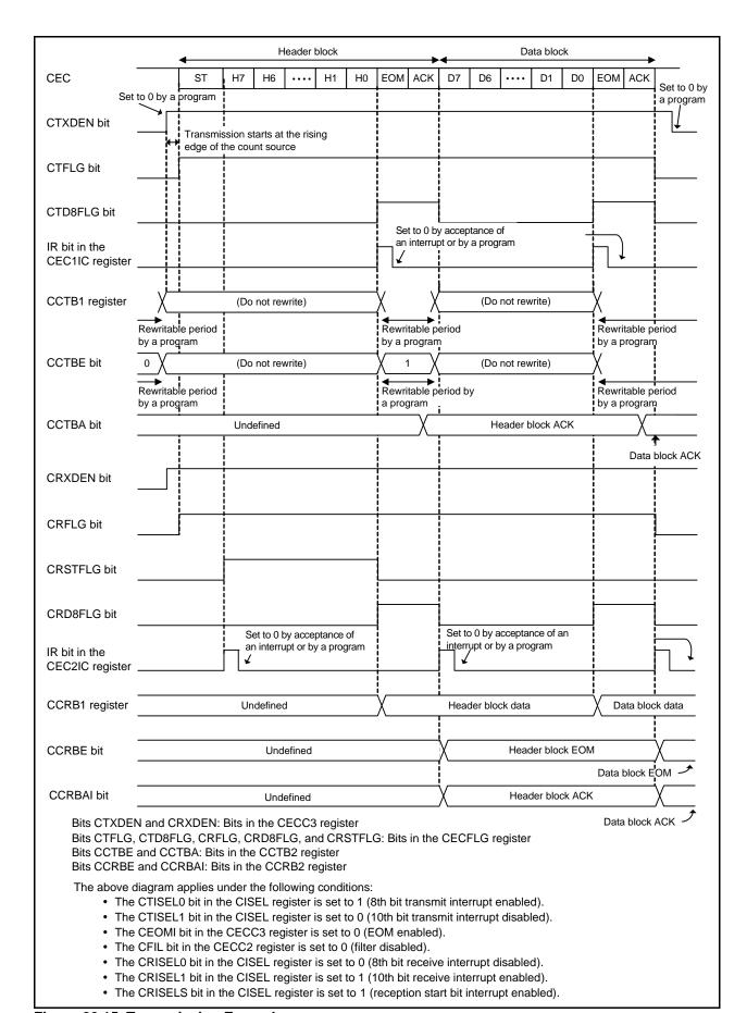
Figure 26.15 Transmission Example
