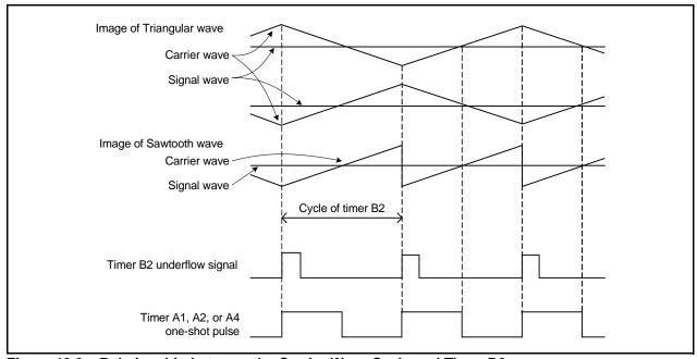
Figure 19.3 Relationship between the Carrier Wave Cycle and Timer B2
