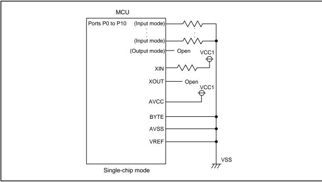
Figure 13.15 Unassigned Pin Handling in Single-Chip Mode
