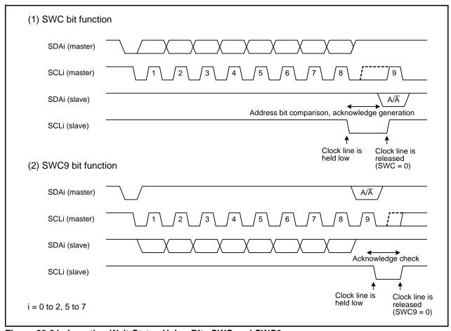
Figure 23.24 Inserting Wait-States Using Bits SWC and SWC9
