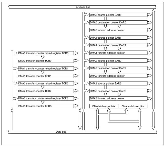
Figure 16.1 DMAC Block Diagram
