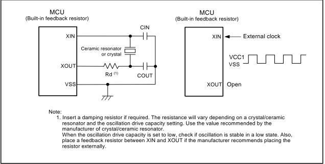
Figure 8.2 Main Clock Connection Example
