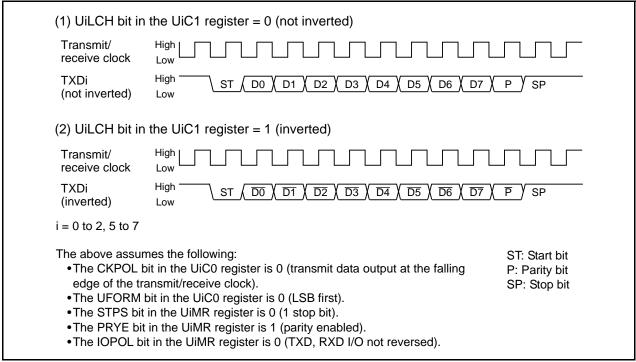
Figure 23.15 Serial Data Logic Switching
