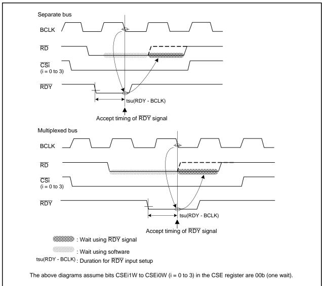
Figure 11.4 Examples in Which Wait State Was Inserted into Read Cycle by RDY Signal
