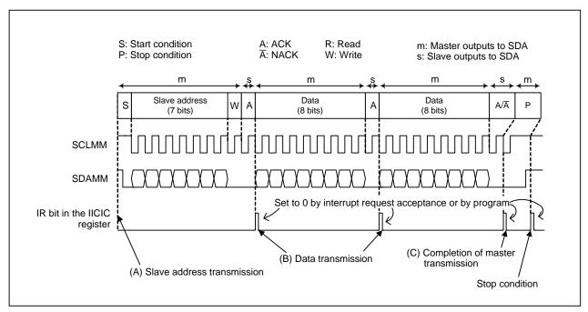
Figure 25.17 Example of Master Transmission
