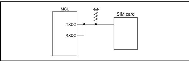
Figure 23.36 Example of SIM Interface Connection
