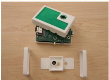
Position the **pitouch-top** part over the Raspberry Pi and angle it down so the SD card slot slips into the proper opening of the pit ouch-part.
