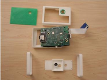
prevent any shorts. Use a short ribbon cable and flip it over to the back of the Pi, covering the ethernet port.
