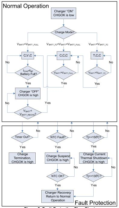
Figure 5: Fault-Protection Flow Chart
