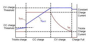
Figure 2: Li-Ion Battery Charging Profile
