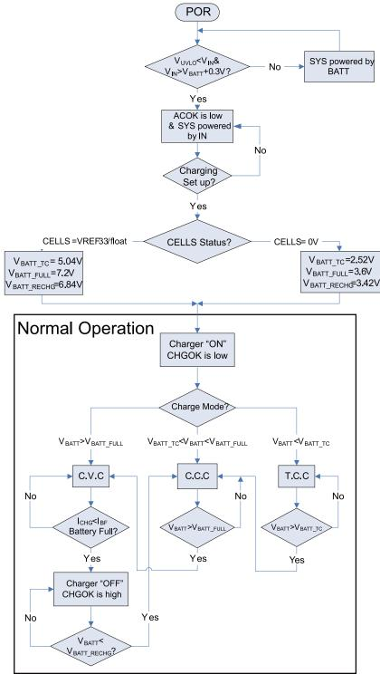
**Figure 4: Normal Charging Operation Flow Chart**
