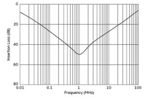
Common Mode Insertion Loss (Typ.)
