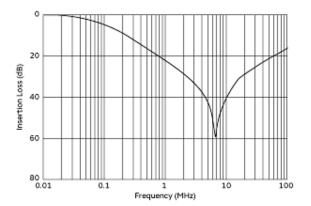
Differential Mode Insertion Loss (Typ.)
