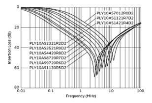
Differential Mode Insertion Loss-Frequency Characteristics
