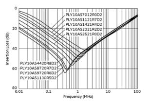
Common Mode Insertion Loss-Frequency Characteristics
