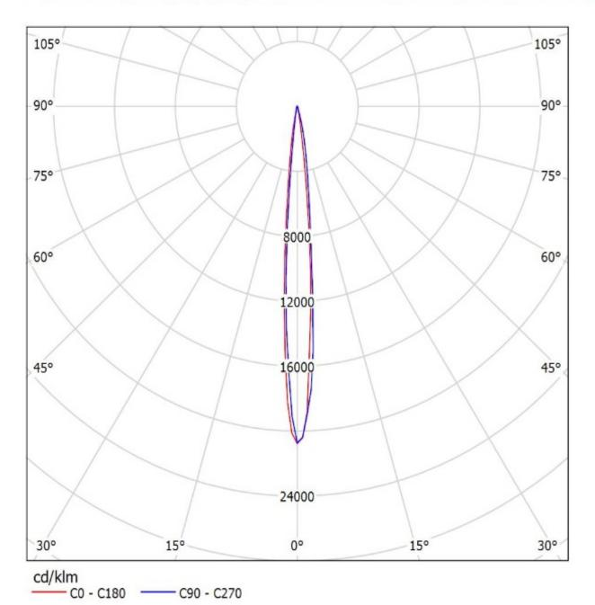
Luminaire: LEDiL Oy FA10886\_TINA-RS\_(Golden\_Dragon+) Lamps: 1 x Osram\_Golden\_Dragon\_Plus\_(LCW\_W5AM-KYKZ-4L8N-Z)\_66.0029Im@250mA\_P=0.785386W\_I=249.9mA NOTE: The typical divergence will be changed by different color, chip size and chip position tolerance. The typical total divergence is the full angle measured where the luminous intensity is half of the peak value.
