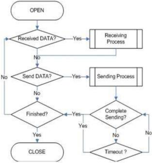
Figure 14 IPRAW Operation Flow
