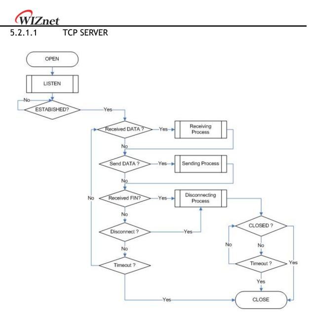
Figure 10 TCP SERVER Operation Flow
