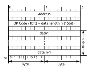
Figure 19 W5200 SPI Frame Format
