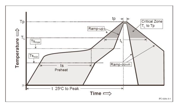
Figure 26 IR Reflow Temperature
