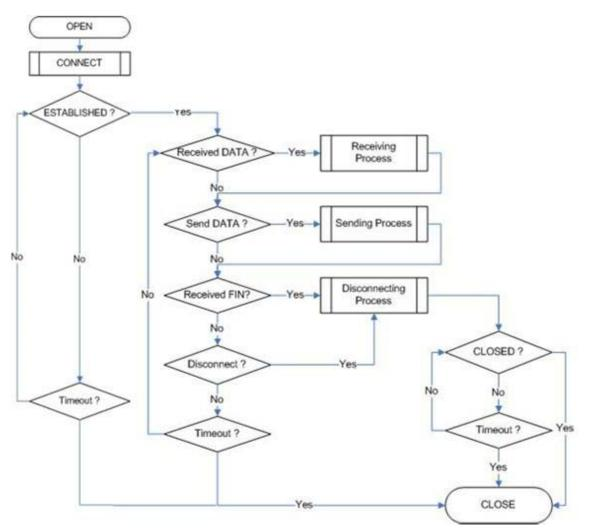
Figure 11 TCP CLIENT Operation Flow
